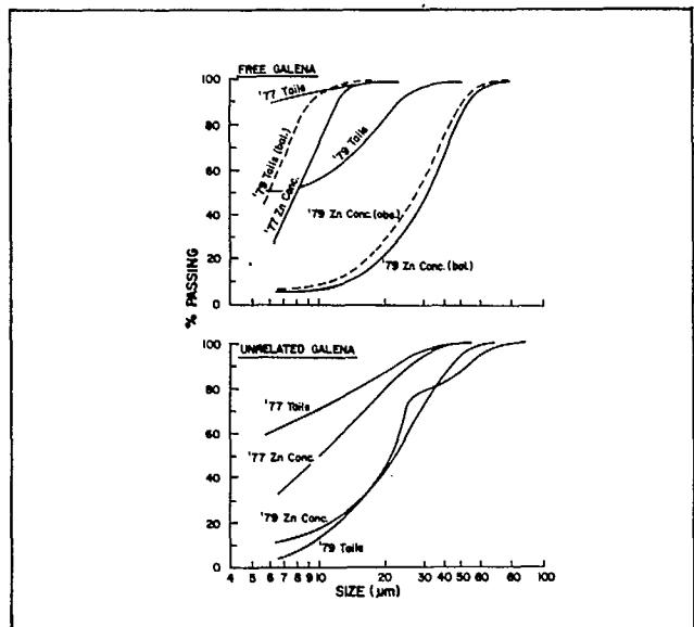
Fig. 5 — Size distributions of free and unliberated galena in tails and zinc concentrates. Plotted as cumulative per cent passing.
