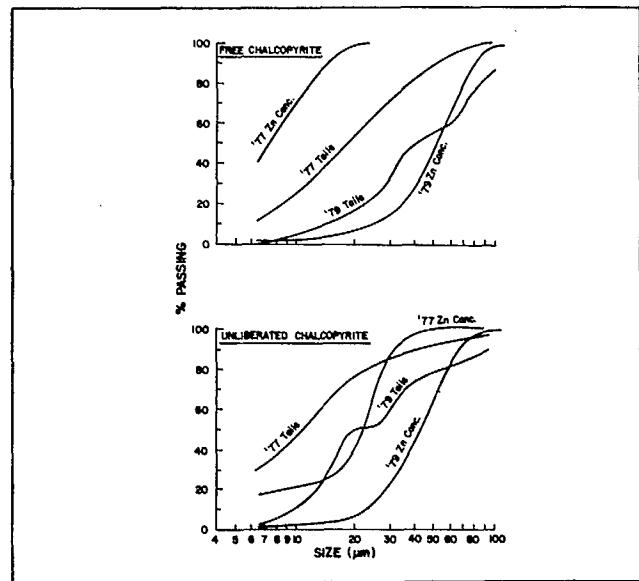
Fig. 6 — Size distributions of free and unliberated chalcopyrite in tails and zinc concentrates. Plotted as cumulative per cent passing.
