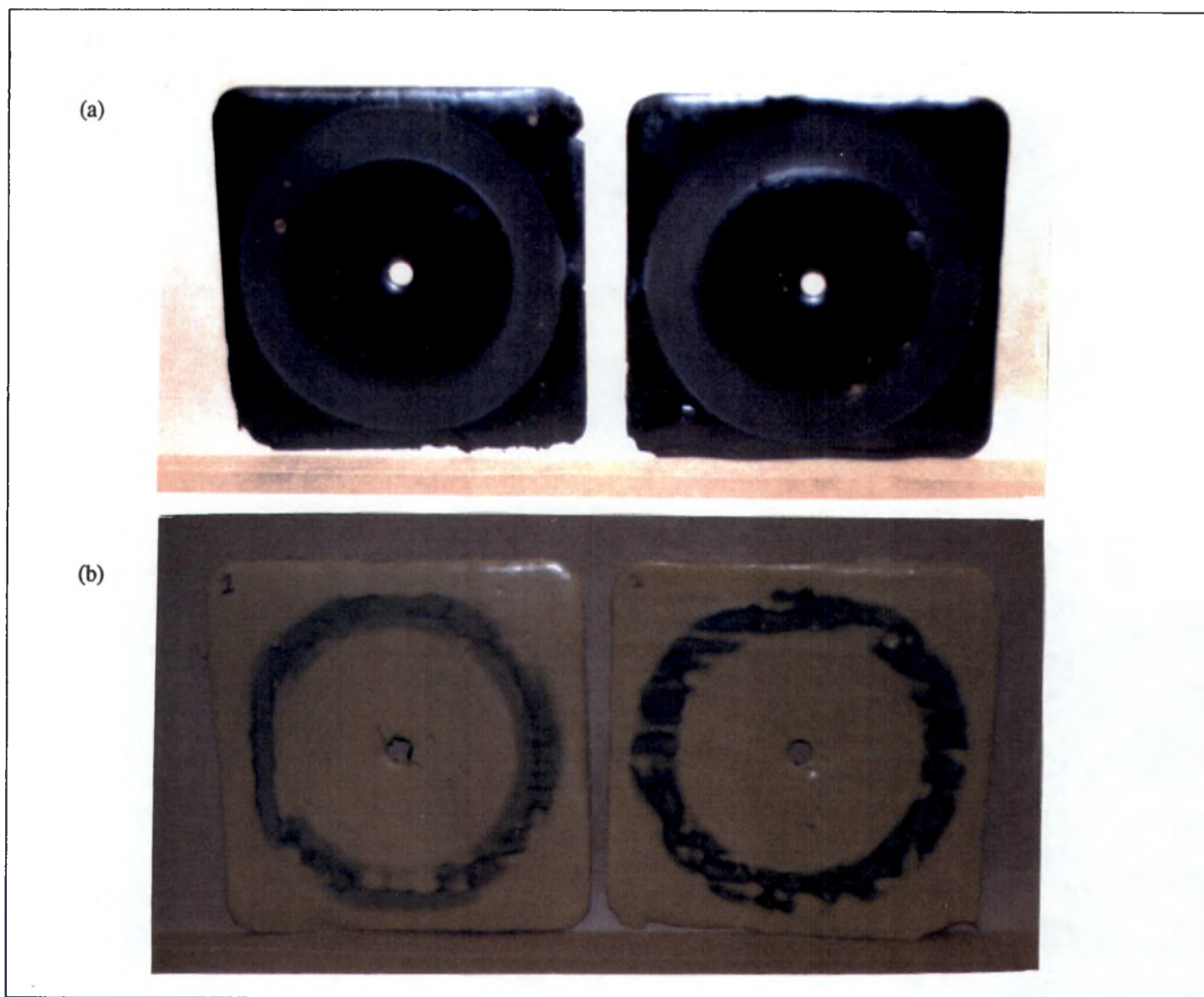
Figure C3. Abrasion Resistance of Free Film Specimens: (a) PDM-4, (b) PDM-5. All samples abraded with CS-17 wheels, 1000g per arm.
