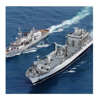
The Joint Support Ships (JSS) will increase the range and endurance of naval task groups, permitting them to remain at sea for significant periods of time without returning to port for replenishment. The JSS will also provide a home base for helicopter maintenance and operation, a limited sealift capability and support to operations ashore. They will replace the Royal Canadian Navy's retired Protecteur-class auxiliary oiler replenishment vessels.
