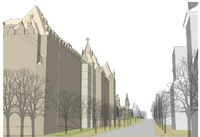
106. Wellington view looking east. The upper floors of the Infill Building are set back to maintain the full visibility of the existing copper roofs
