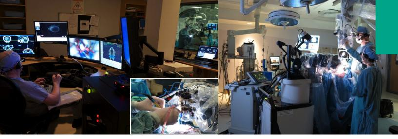
The microsurgical robot neuroArm merges machine technology derived from the International Space Station's Canadarm2 with intraoperative imaging [Courtesy: Project neuroArm, University of Calgary]
