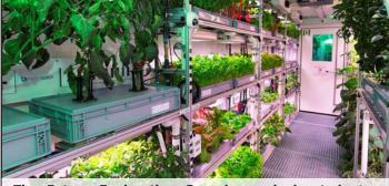
The Future Exploration Greenhouse is located at an Antarctic research base. The University of Guelph and other international partners are using this test facility to develop plant cultivation technologies for space [Courtesy: DLR, 2017]
