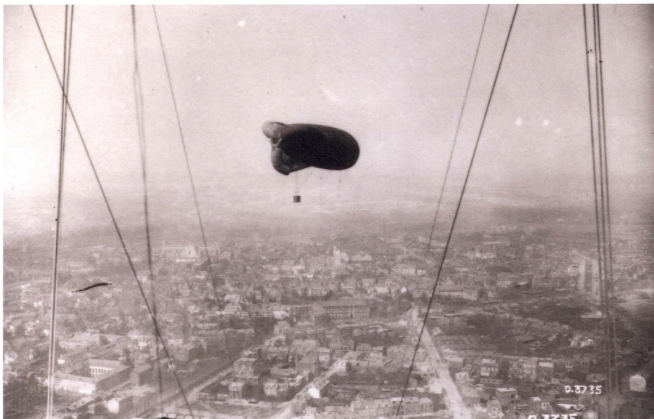
This kite balloon over Arras, France, helped mapmakers to collect vital target information on the German lines. A heavy metal cable tethered the balloon to a ground-based mobile winch that would haul the highly inflammable hydrogen-filled balloon and its observer back to the launch site once it attracted enemy fire. Canada, Dept. of National Defence, A kite balloon over Arras , 1917, PA 003651
