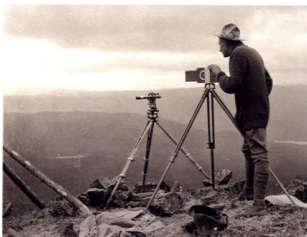
A surveyor adjusts his topographic camera during field trials in the Rocky Mountains. To the left is the theodolite that was used to calculate the bearing (or angle) to other mountain tops.
