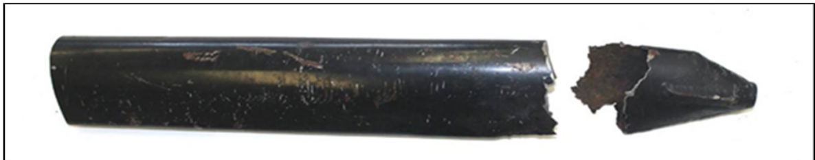
Figure 2. Damage on the upper half of the left main spar wing lift strut assembly (Source: TSB)
