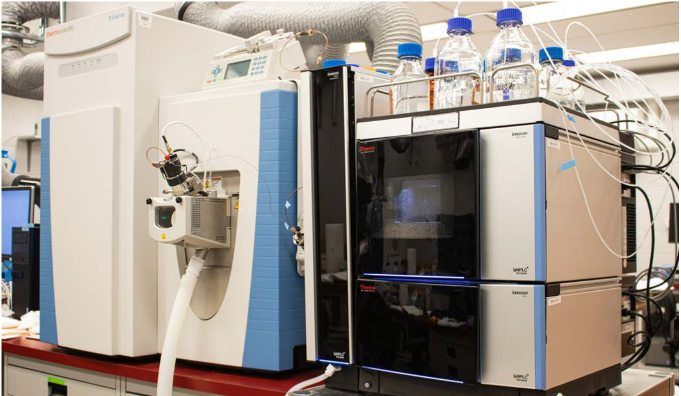
Figure 3 We use a liquid chromatograph high-resolution mass spectrometer to analyze pesticides in grain
