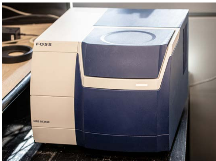
Figure 2 Benchtop NIR spectrometer used for predicting oil and protein content in soybeans
