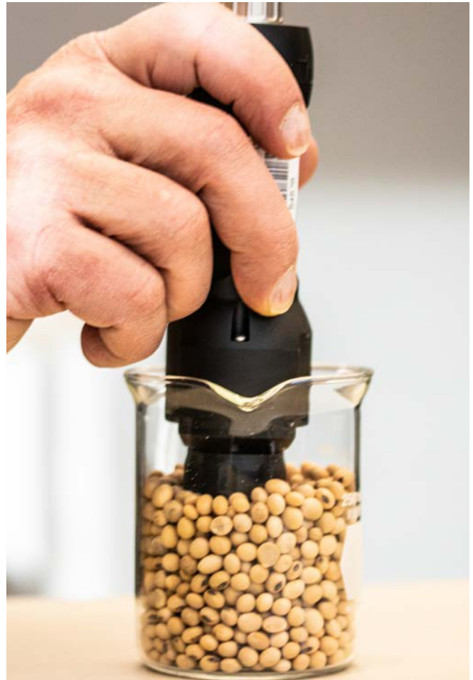
Figure 3 Handheld NIR spectrometer used for predicting oil and protein content in soybeans
