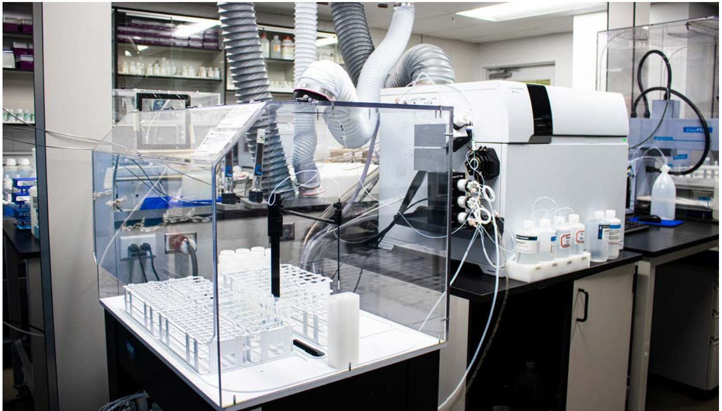
Figure 1 Our program uses this inductively-coupled mass spectrometer with robotic autosampler to analyze trace elements, including heavy metals such as lead and cadmium, in grain
