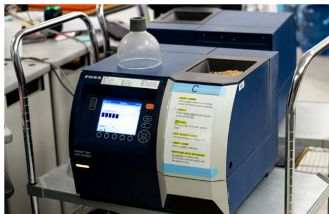
Figure 1 A Foss Infratec™ 1241 Grain Analyzer used to analyze protein content in whole kernels of wheat and other cereals
