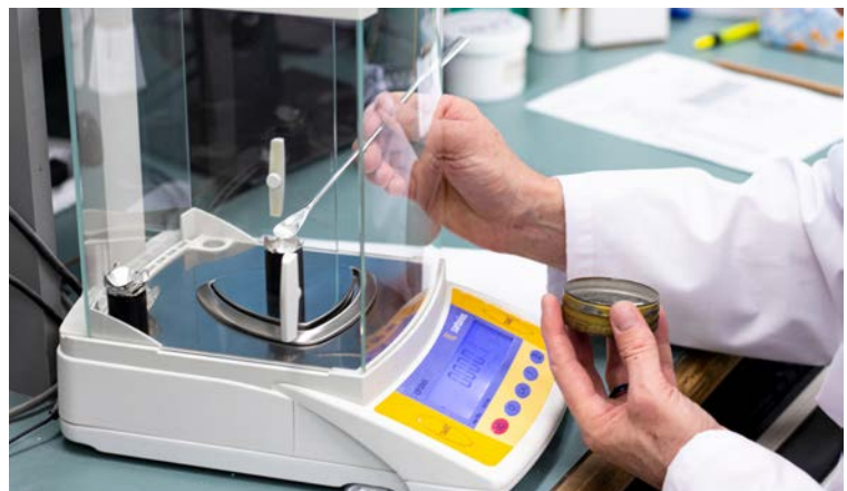
Figure 4 A sample being weighed for combustion nitrogen analysis
