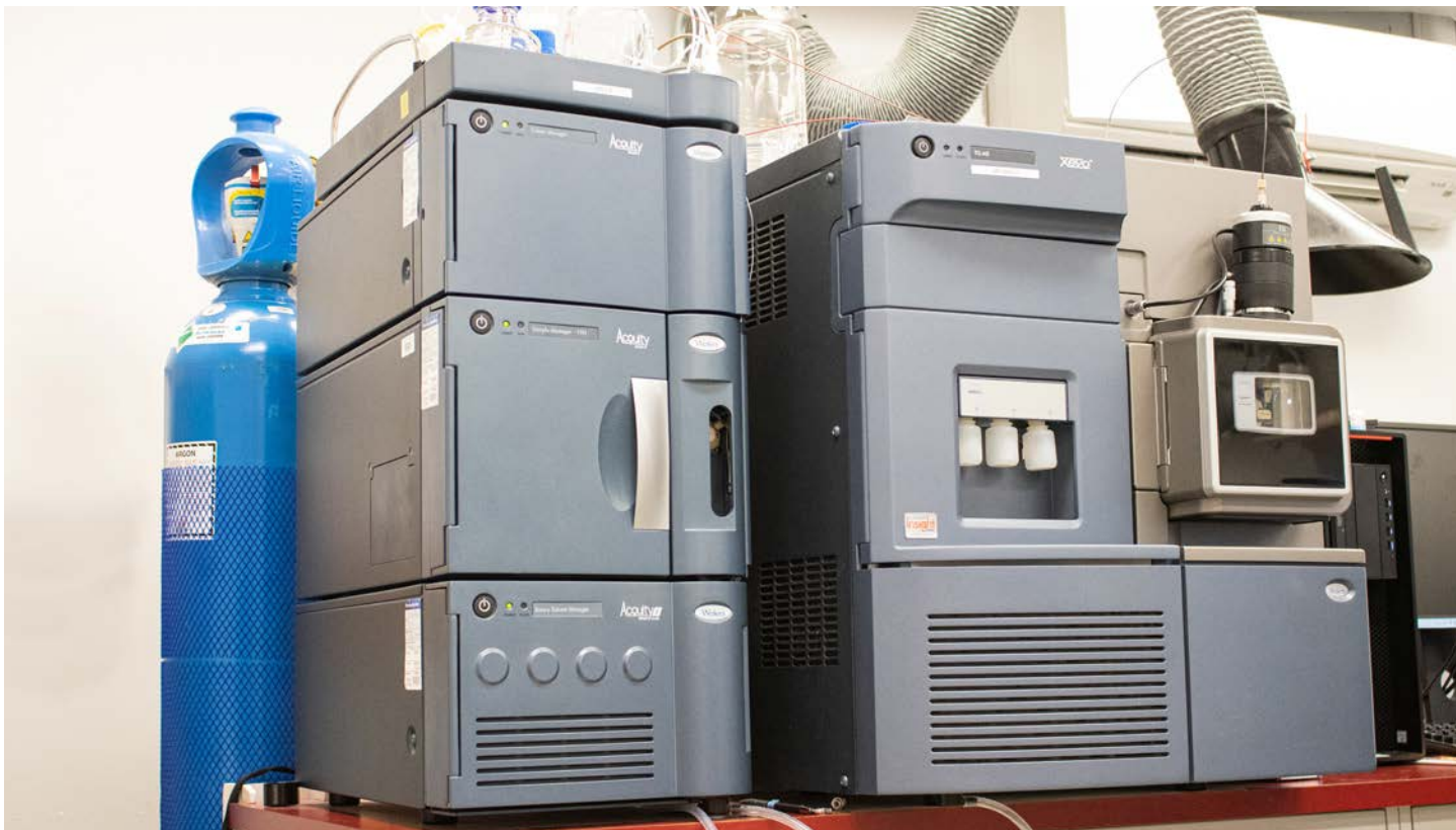
Figure 5 We use this liquid chromatograph tandem mass spectrometer to analyze mycotoxins in grain. This technology allows us to measure concentrations in the parts per billion range.
