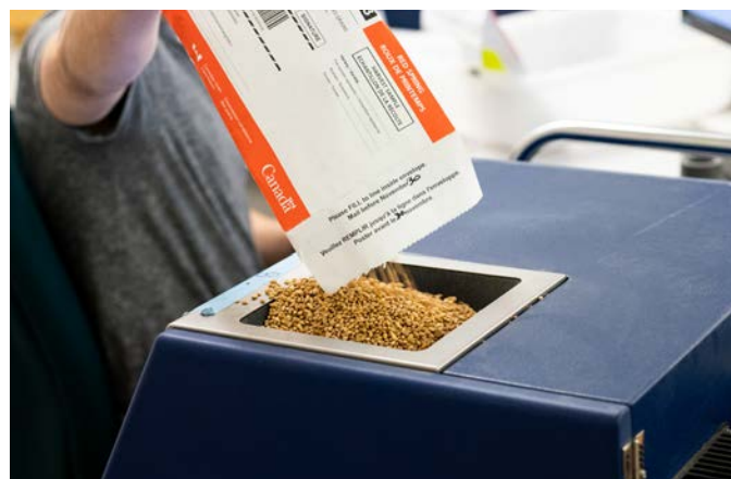
Figure 2 A grain producer's Harvest Sample Program contribution being added to a Foss Infratec™ 1241 Grain Analyzer
