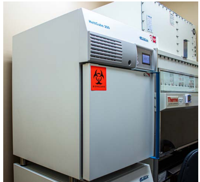
Figure 1 Incubator used for growing microbes in a temperature controlled environment
