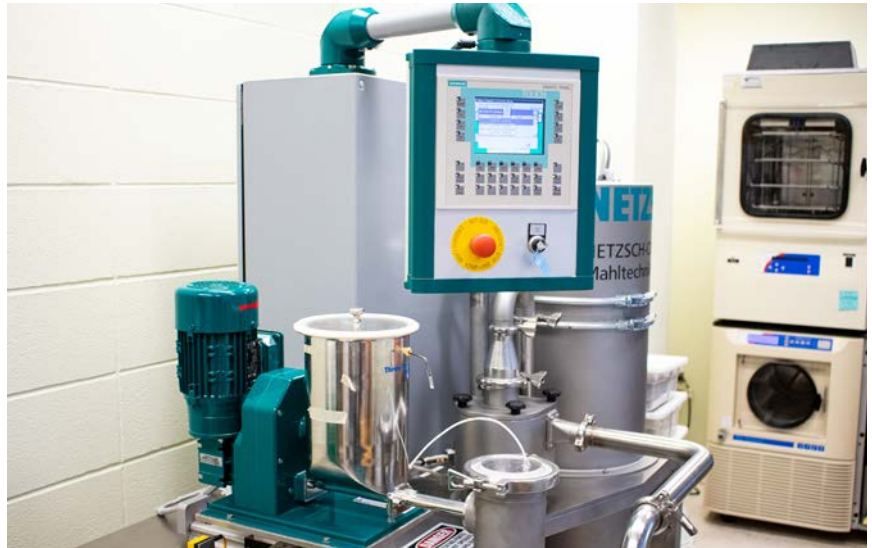
Figure 2 Laboratory air classifier for separation of pea flour into protein-rich and starch-rich fractions
