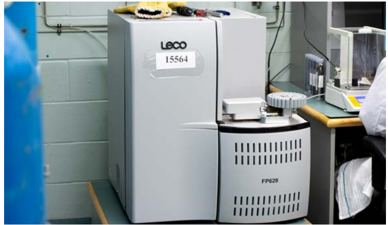
Figure 3 Leco FP-628 used for combustion nitrogen analysis (CNA) to measure protein in ground grain, pulses and oilseeds
