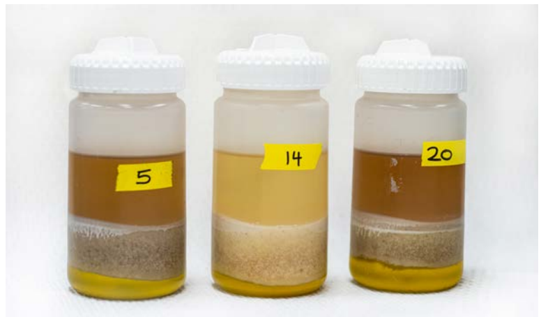
Figure 4 Cereal grain samples being processed for the analysis of pesticides. The pesticides are in the top layer with water. The ground grain sample is the middle layer. A solvent that removes other grain components and prevents them from interfering with the analysis is the bottom layer
