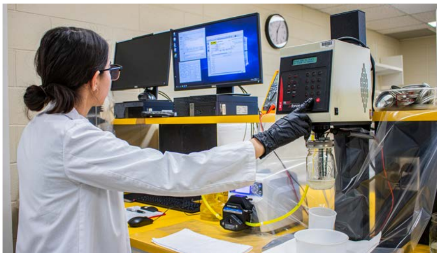
Figure 1 The apparatus we developed to measure oil emulsifying capacity in pulses
