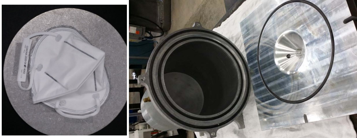
Figure 2. N95 respirator mounting and testing chamber. (Left: N95 respirator glued on a disc with a 90 mm diameter hole in the middle. Right: respirator-testing chamber, open.)
