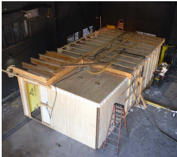
Figure 3 Outside view of the test compartment
