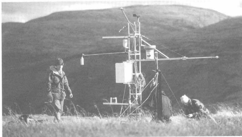
Figure 6 Ultrasonic snow-depth sensor, Wolf Creek, Whitehorse, Yukon.
