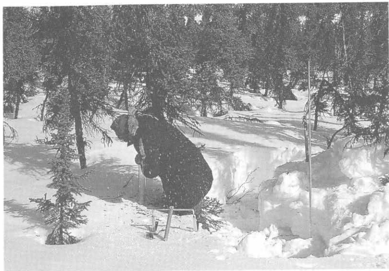
Figure 9 Snow sampling tube and scale, Inuvik, N.W.T.
