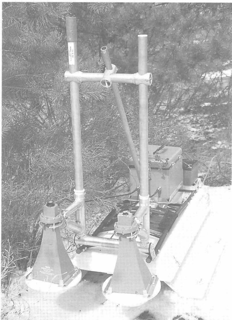
Figure 8 NHRI's microwave (FMCW) radar unit.
