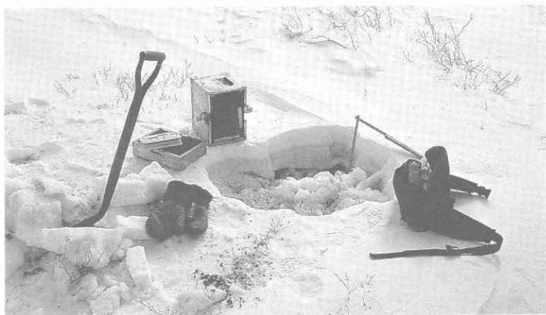
Figure 7 Gravimetric sampling of snow water equivalent, Inuvik, N.W.T.
