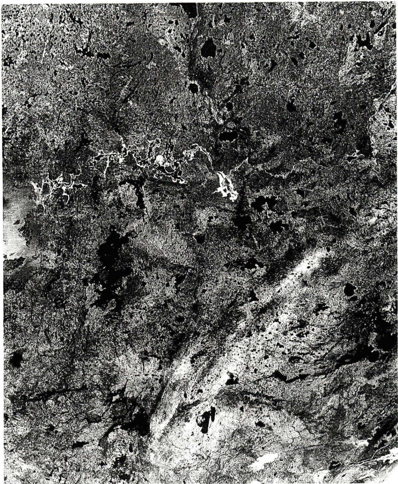
Landsat MSS color composite (bands 4, 5 and 7) of the lower Churchill River. Image was acquired June 25, 1981. Altered turbidity and water levels can be identified in this post-diversion image.
