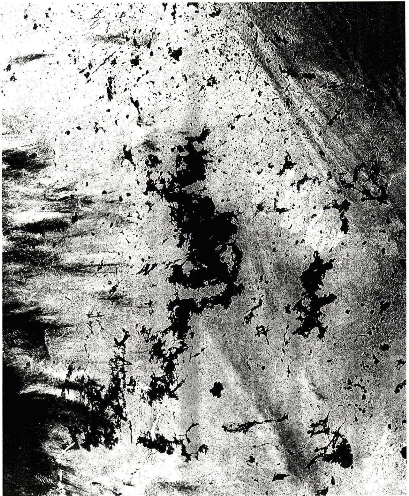
Landsat MSS (band 6) winter scene of Southern Indian Lake. Image was acquired May 12, 1984. The breakup pattern is consistent with Plate 11. Open water is white (negative image). Landsat MSS winter scenes are presented in Plates 9-12.
