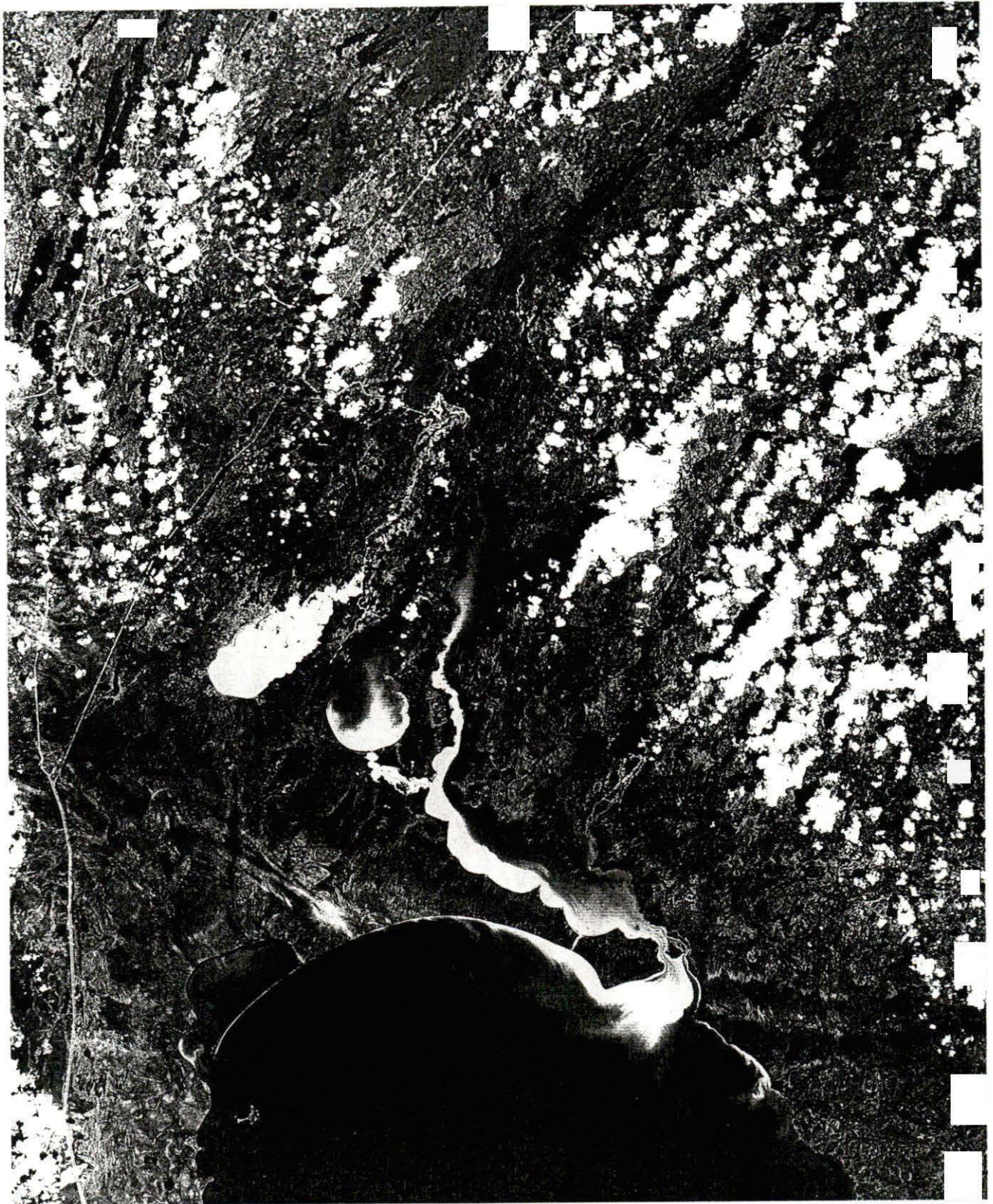
Landsat MSS color composite (bands 4, 5 and 7) of Outlet Lakes. Image was acquired July 4, 1974. Water turbidity patterns (lighter colored water), hydro electric structures (linear channels) and vegetation clearing (light color along lake shores and rivers) are visible.
