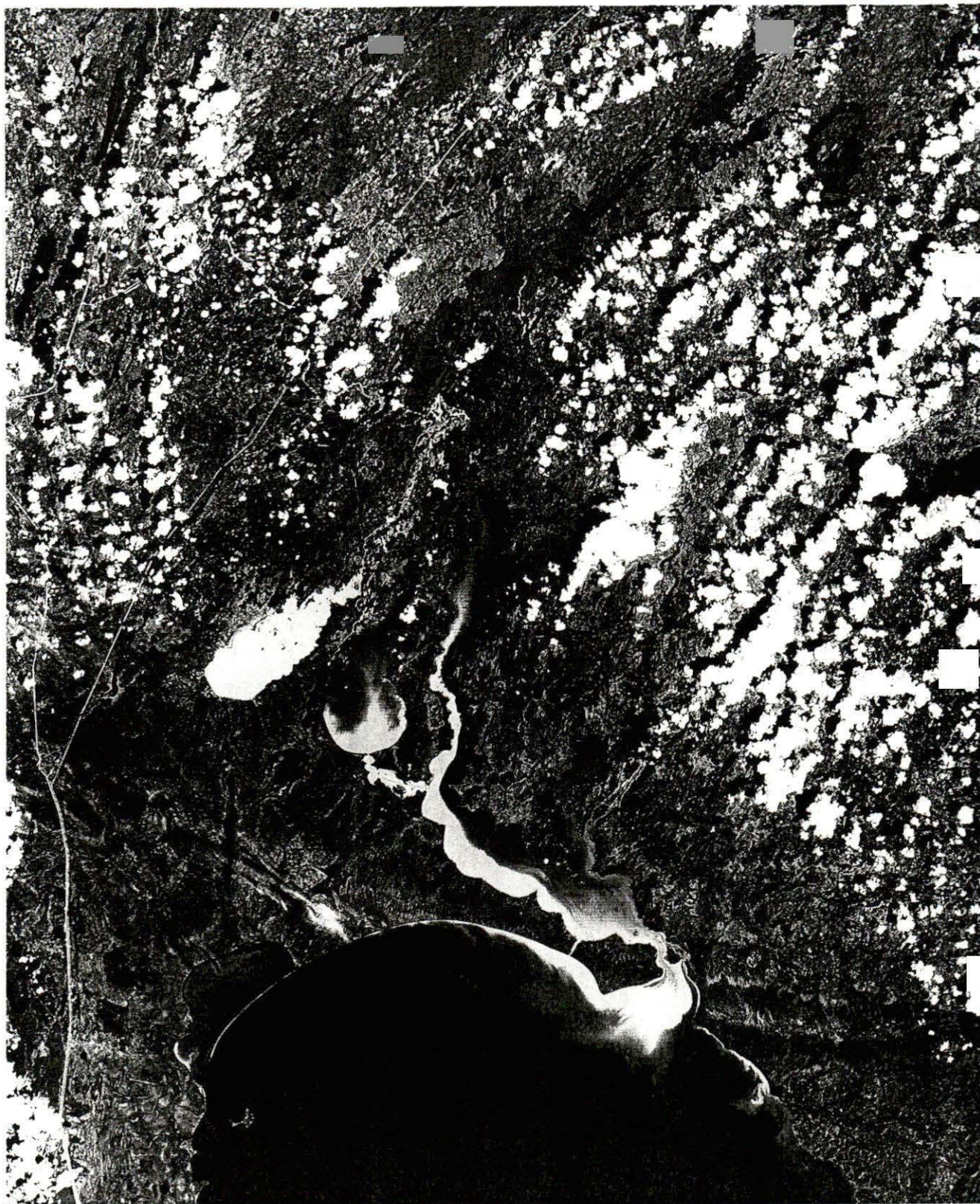
Landsat MSS color composite (bands 4, 5 and 7) of Outlet Lakes. Image was acquired July 4, 1974. MSS and TM (Plate 13) have the same spatial coverage but TM has improved pixel and radiometric resolution.
