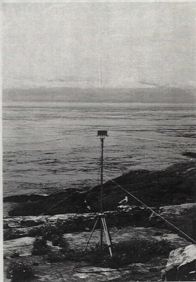
Figure 2.2 View of Race Rocks (upper photograph) from the north. The SeaSonde hardware was installed in the light tower. The transmit and receive (lower photograph) antennas were deployed on the south side of the island.
