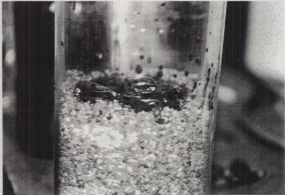
Figure 4. Tarry residue on the surface of a coarse-sand test column. Note the “ropey” nature and viscous consistency.
