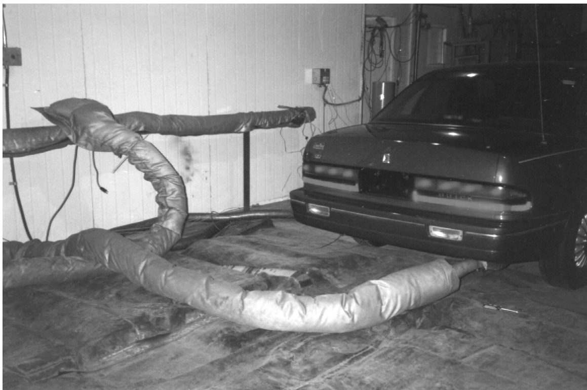
Figure 2. Vehicle in testing position on chassis dynamometer (back view).
