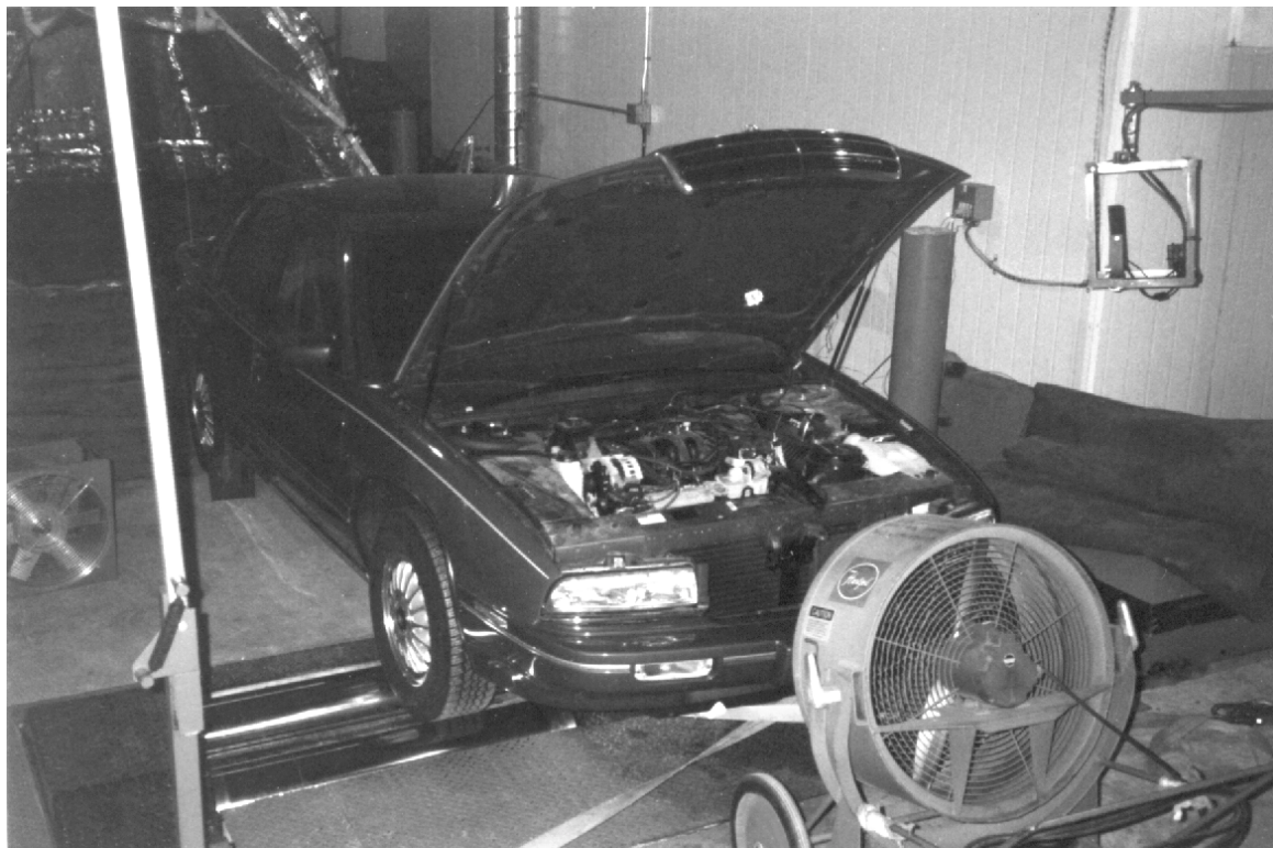
Figure 2. Vehicle in testing position on chassis dynamometer (back view).
