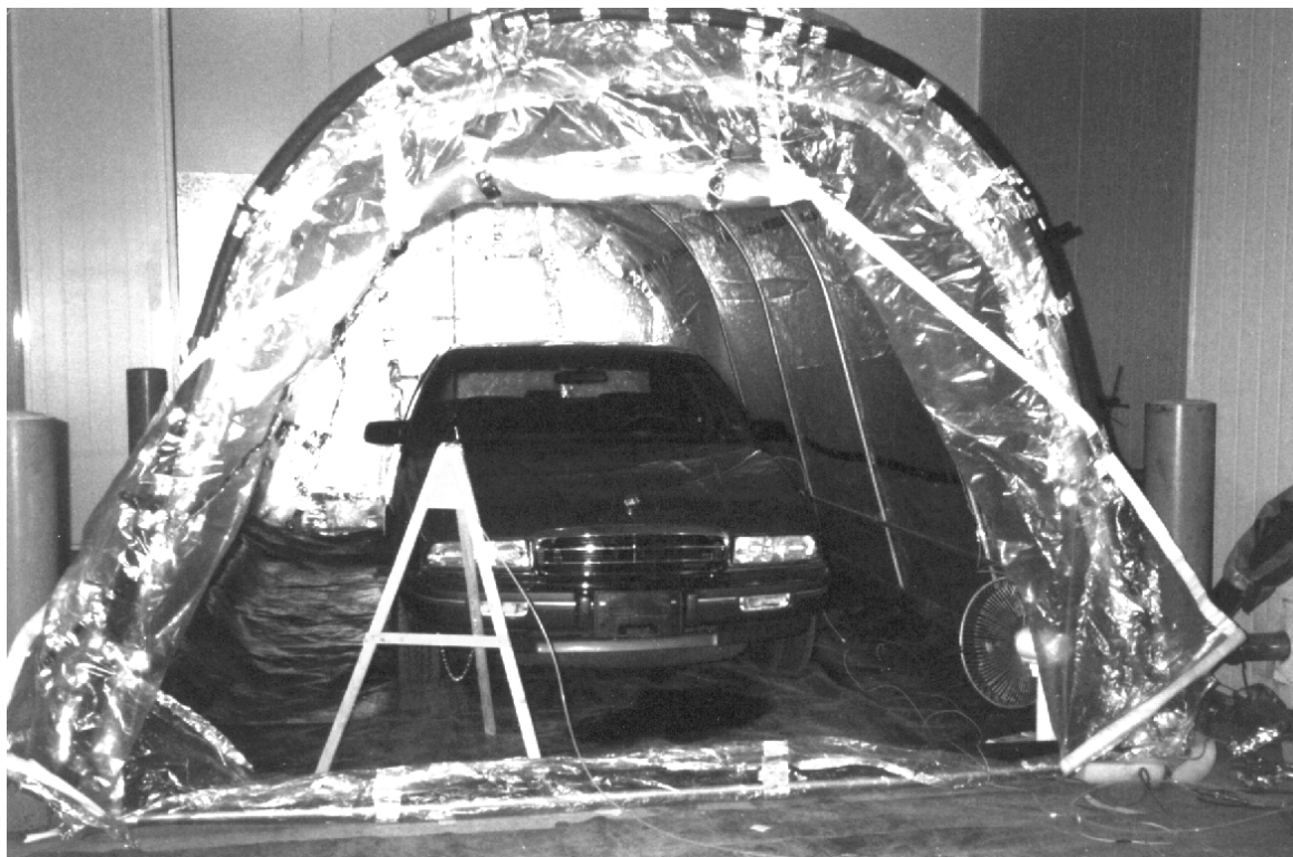
Figure 4. Test vehicle in position inside the SHED.
