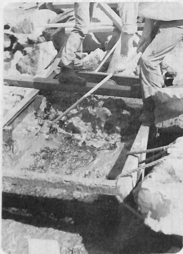
Figure 10. Partial pipeline diversion monitoring facility. Note the unmanageable flow and heavy debris obscuring any specimens.
