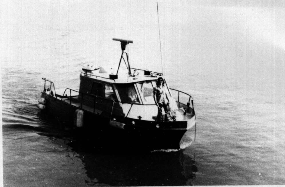
35 FOOT STEEL HULLED SURVEY LAUNCH , ONE OF TWO USED ON SURVEY
