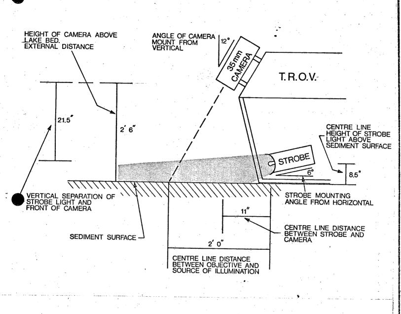
Camera : EG&G model 205 Lens : 35 mm focal length, f4.5, water corrected Aperture setting : f22 Shutter speed : 1/50 second Focal distance setting : 3 feet Depth of field at settings : 2'2" to 4'9"
