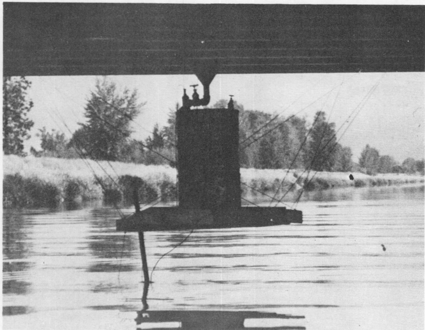
Figure 2A. Platform used to release dye into the Okanagan River at the Highway 97 bridge. Barrel with the constant head siphon is mounted on the platform.
