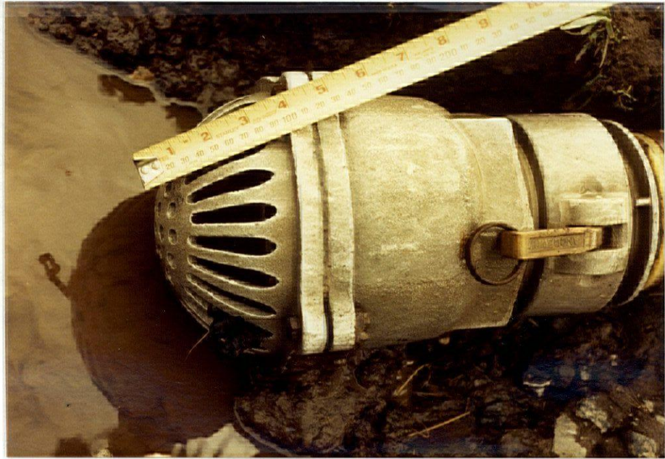
PLATE 79 - A typical water intake screen which exceeds the recommended mesh opening size of 0.1 inch (25 mm). Intakes, such as this, may entrap small fish (km 128.3, Hwy. 2).
