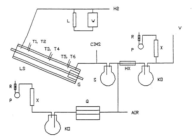
To represent the destruction efficiency obtained using the boiler and reactor combined, a second sidestream is drawn from the main stream immediately after the scrubber flask. This is drawn through a quartz tube furnace (Q) along with air metered in through a valved rotameter. A water knockout flask dries the incinerated gas stream prior to it passing through an XAD2 resin tube system.
