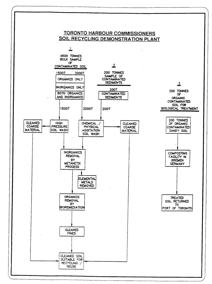
slurry will be returned to our demonstration plant where we will further treat the contaminated slurry. To test the soil scrubbing wash process we will lease a wash facility from Bergmann U.S.A. which will wash up to 50 tonnes per day on-site and will be fully integrated with the two following soil cleaning technologies. Up to 3000 tonnes of contaminated soils will be washed by the Bergmann wash plant which will remain on-site for about four months.
