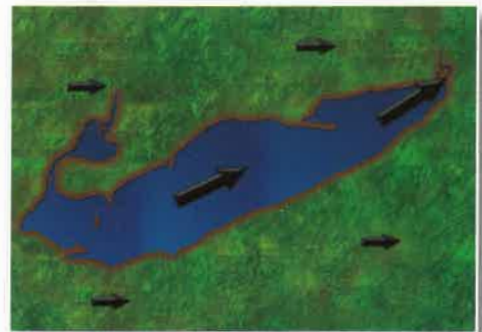
Large-scale channelling and funnelling on Lake Erie. Note direction of winds along the lake axis and stronger winds at the east end.
