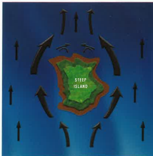
Corner effects around a steep island. Note that winds increase on both sides of the island, but are slightly stronger on the left than on the right. Also, note the gusty lee winds behind the island.
