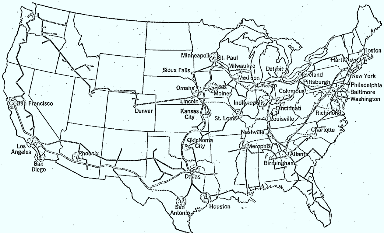
FIGURE 6. The proposed MCI carrier network (color) and the Datran data communication system (black).
