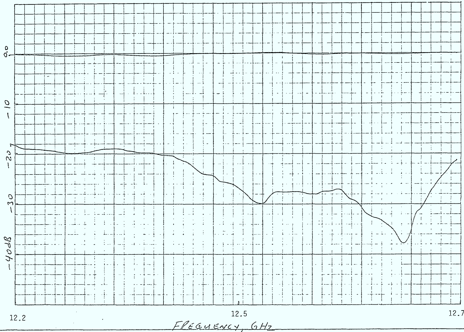
Figure 3-13: Measured return loss of the feed.
