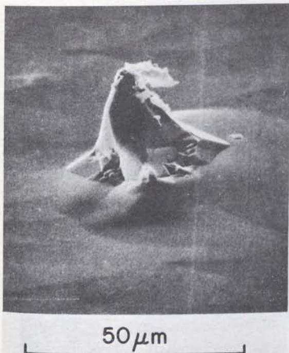
(a) SEM micrograph (emissive mode) of growth pyramid
