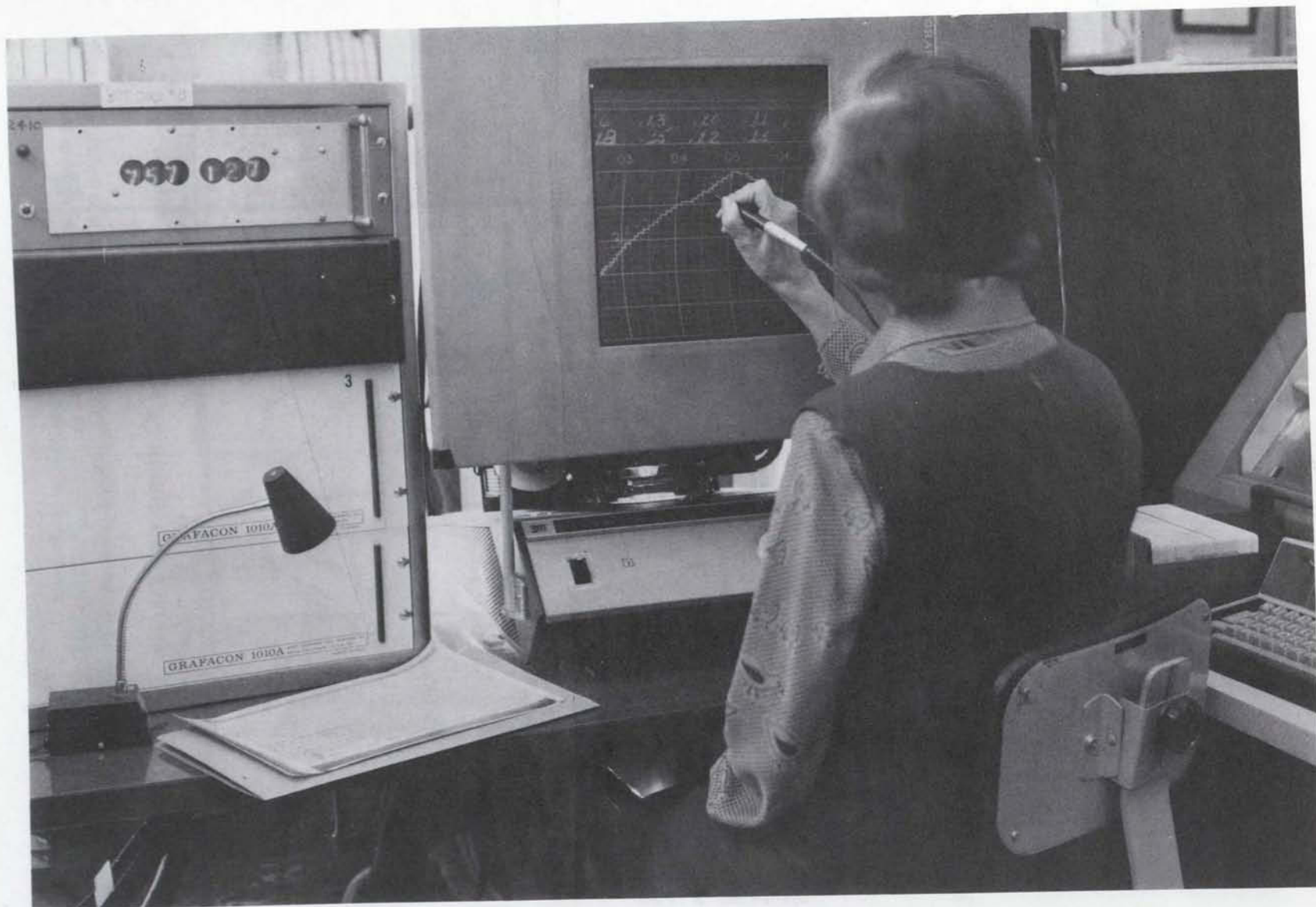
Figure 3. Digitizing the enlarged trace of a tipping-bucket rain chart
