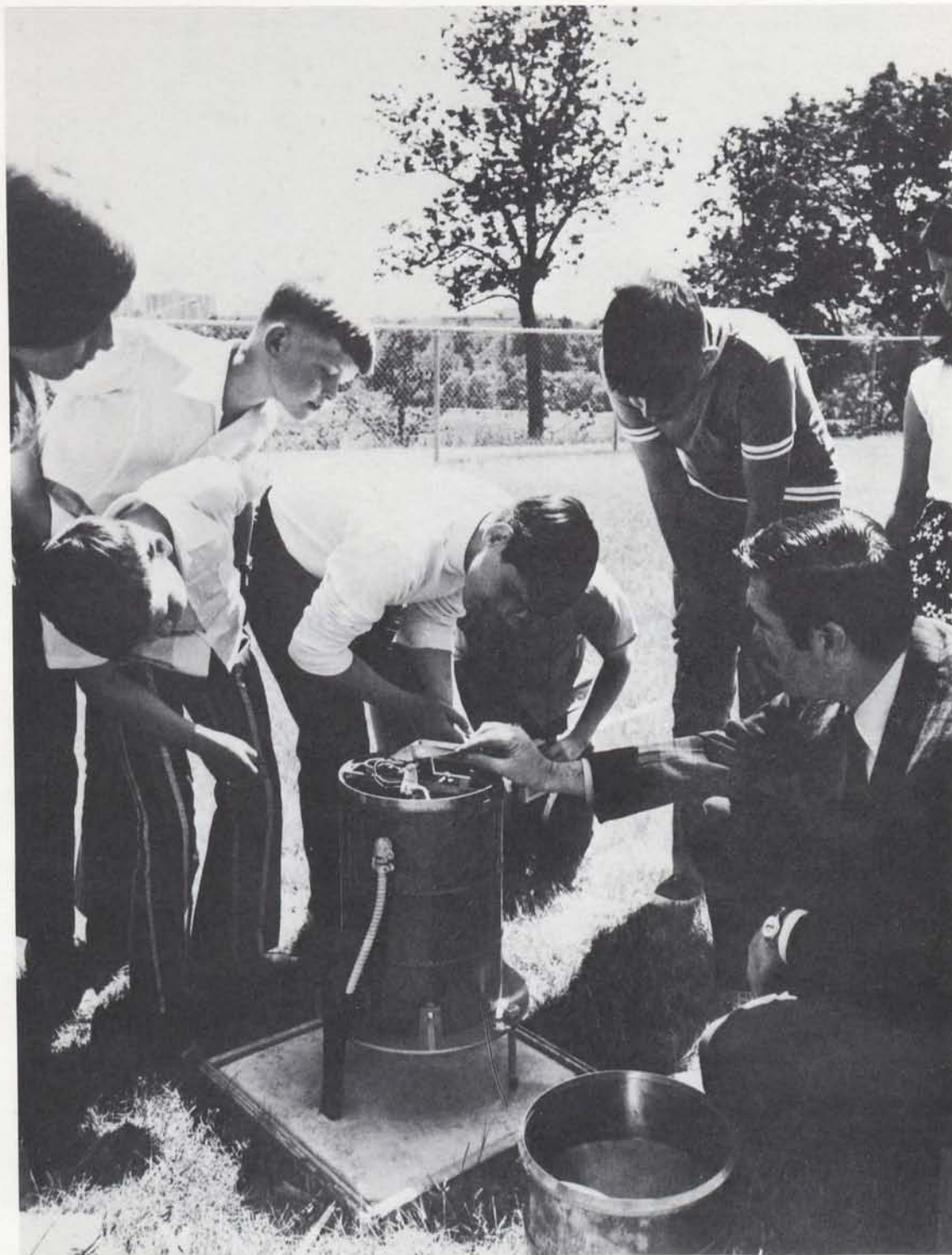
Examining the tipping-bucket mechanism inside a recording rain gauge. The rain-collecting area is defined by the cylindrical funnel mouth, seen here lying in the foreground. The data analyzed in this report were derived from records taken at locations across Canada with a network of instruments of this type. (Photo courtesy Fisheries and Environment Canada).
