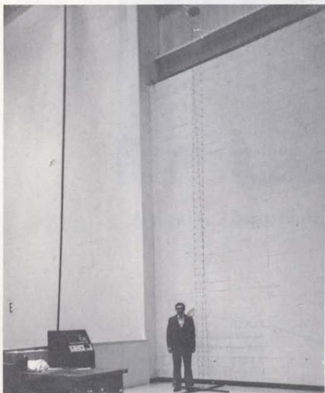
Figure 1. 7.6 Meter CRC Astromast in Fully Deployed State
