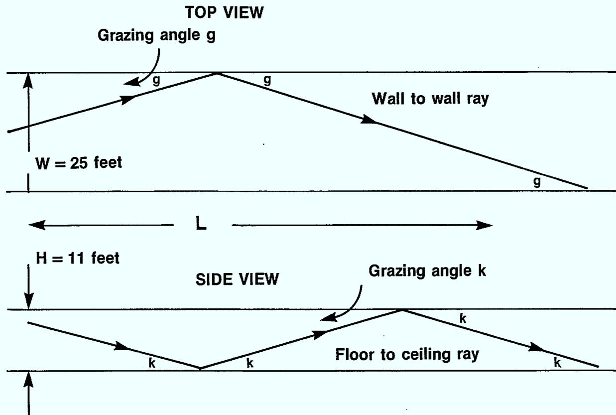
FIG. 1A RAYS IN WAVEGUIDE
