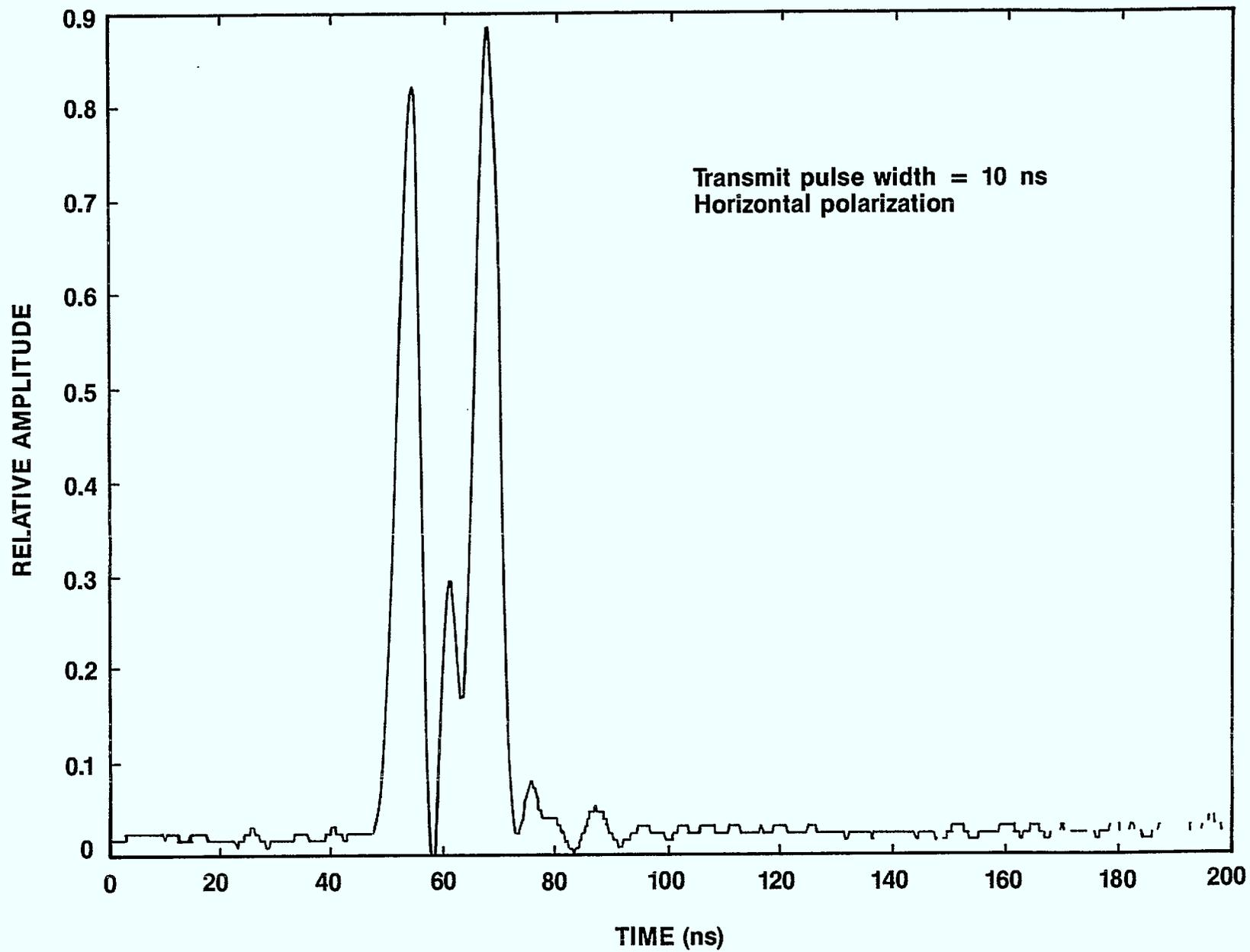
FIG. 5 IMPULSE RESPONSE IN POTASH TUNNEL
