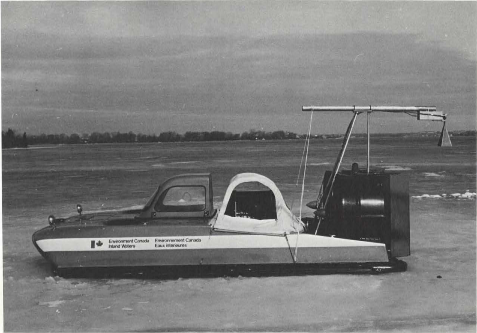
Figure 27. Radar Mounted on ACV
