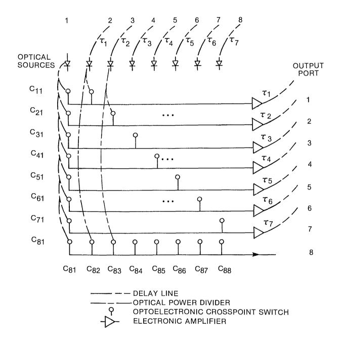
Figure 3. A Submatrix for Loop Filtering which Involves Single Delay Line Only.
