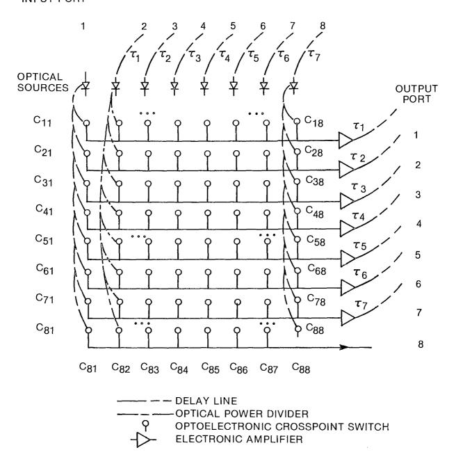
Figure 1. An 8x8 Reflex Optoelectronic Switching Matrix (ROSM).
