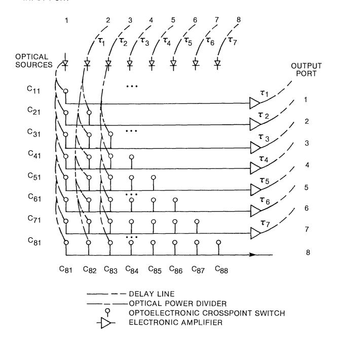
Figure 2. A Submatrix for Delay Generation.
