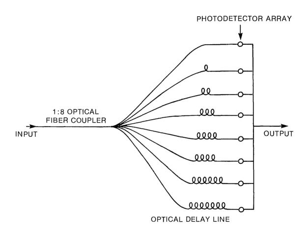
Figure 5. A Submatrix for Word Detection, Integration and Digital to Analog Conversion.
