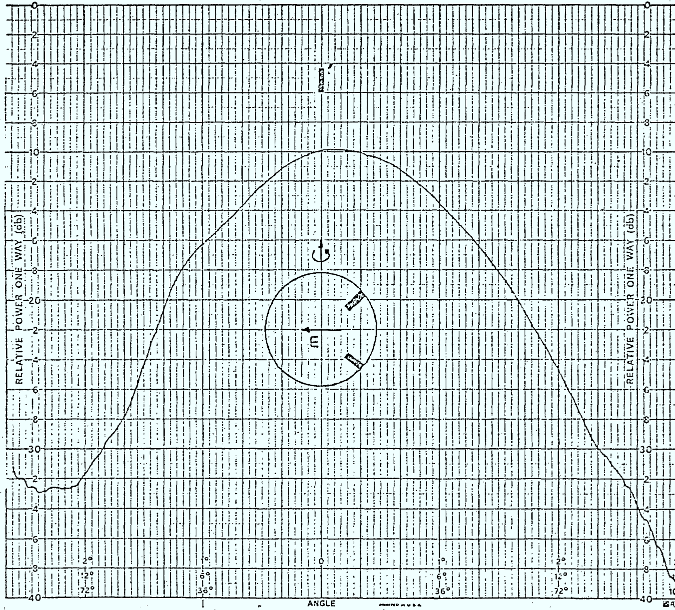
E-plane measurements for vertical polarization with the diagonal screws different from Fig. H'.
