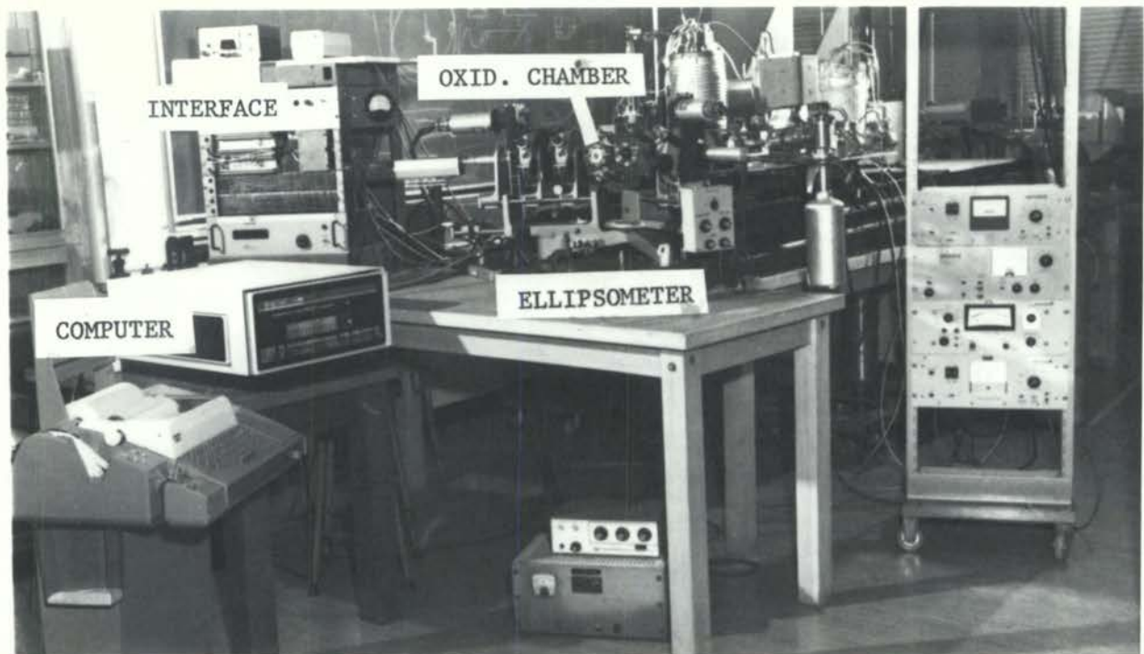
Fig. 1 a) Overall view of oxidation chamber and computer operated automatic balancing ellipsometer
