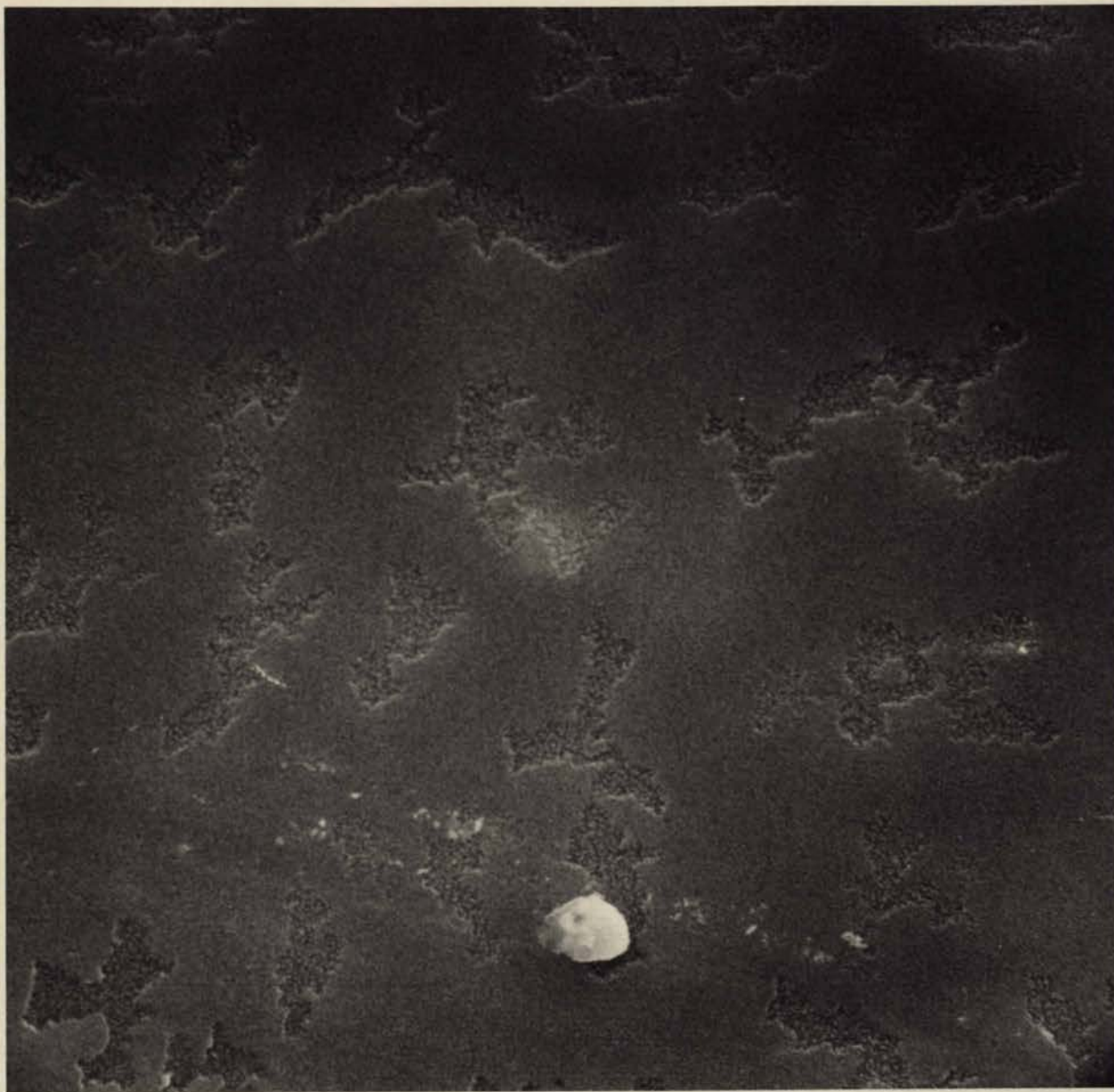
Fig. 2 b) S.E.M. micrograph (2000X) of a thermally etched silicon substrate.
