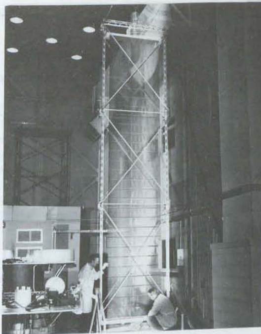
A specially made adjustable holding fixture designed and constructed by CRC Technical Services capable of locating and holding the CTS solar array for inspection and environmental testing purposes.
