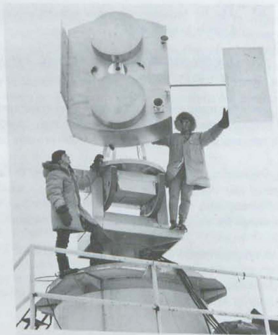
This "Mock-Up" of the C.T.S. was made by Technical Services to check the effect of the spacecraft configuration on the Antenna Pattern of the SHF Beacon.
