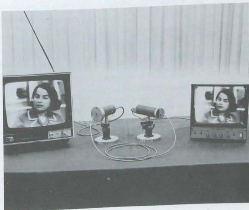
TV baseband transmission through optical fiber-waveguide bundle.
