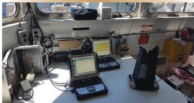
Figure 3. The Puma system’s hand-held controller with mission planning and maintenance laptops on the bridge of an MCDV.
