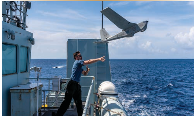
Figure 2. A Puma RPAS being hand-launched from a Kingston -class MCDV.
