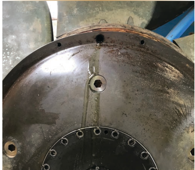
Oil can be seen draining out of the uppermost propeller blade's Prairie Air inlet tube.
