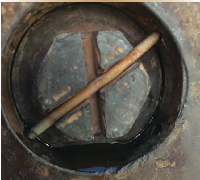
The “ahead” chamber drain plug, showing signs of oil weeping, had backed itself off by a quarter turn.
