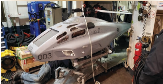
Figure 6. The V-200 aboard a frigate. The custom-built track system was designed by QinetiQ Target Systems to traverse the aircraft from the torpedo magazine into the hangar.
