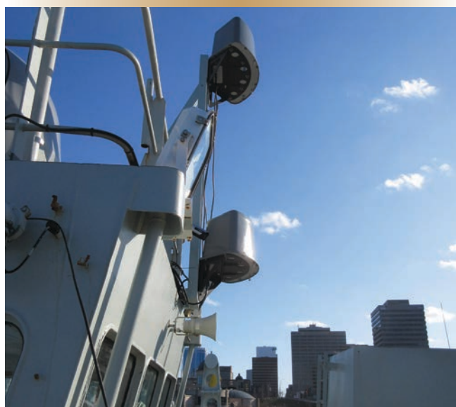
Figure 4. The MCDV superstructure antenna arrangement for the Puma RPAS went through several iterations of development, design and integration to achieve a best fit.
