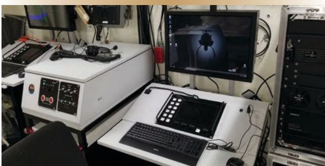
Figure 8. The temporary V-200 control station installed in the CSE technician office aboard a frigate.
