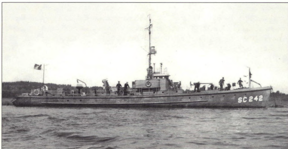
The USN submarine chaser SC 242 spent the summer of 1918 escorting convoys from Sydney, Nova Scotia. At 110 feet long, the wooden sub chasers had a top speed of sixteen knots when fully loaded. In addition to a 3-inch short-range 23-calibre gun, it also carried depth charges. SC 242's "Y" gun, which fired charges off either side, is visible between the three sailors at the rail and the chaser's stern. (DND CN 3279)
