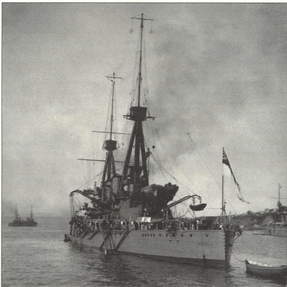
The battle-cruiser HMS Indomitable at the Quebec Tercentenary on 23 July 1908. As conceived by First Sea Lord "Jackie" Fisher, the battle cruiser's eight 12-inch guns and cruiser-like speed would allow it to sweep the world's shipping lanes of all enemy cruisers. (LAC PA-124708)
