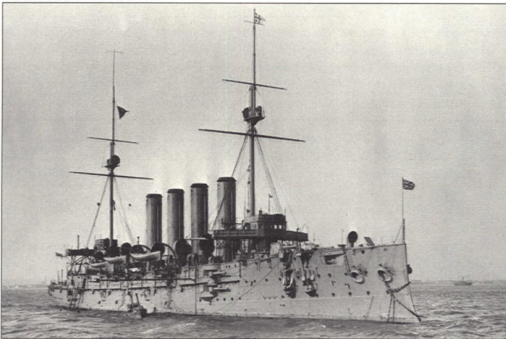
The 11,000-ton Diadem-class cruiser HMS Niobe carried sixteen 6-inch guns, twelve 12-pounders, five 3-pounders and two 18-inch torpedo tubes. (DND CN 6732)
