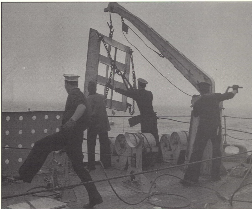
Minesweeping gear was a complicated apparatus whose operation was strenuous, to say the least. Here sailors are lowering the multi-plane "Kite" overboard; the paravane is already in the water. Note the depth charges, as minesweepers were an integral part of the war against the U-boat. (DND NP 1415)
