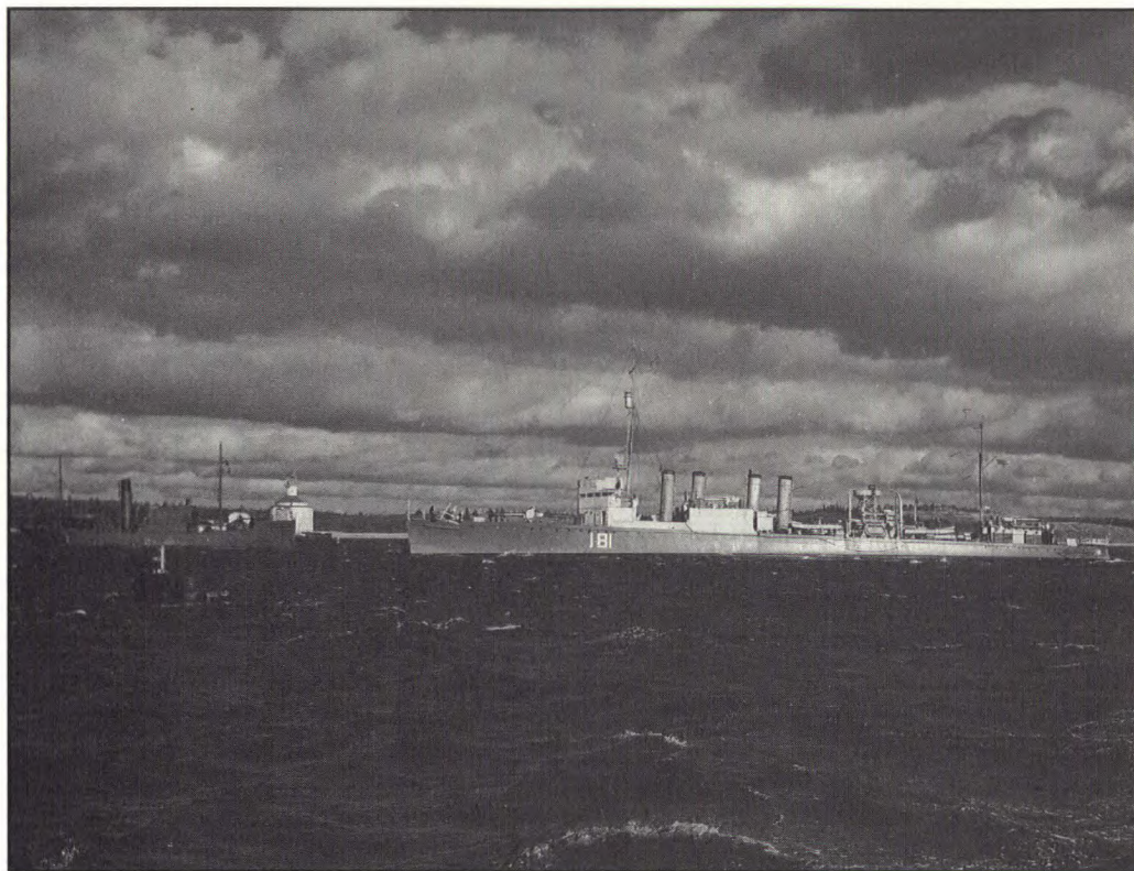
HMCS St Croix , lost to U 87 . Note the four funnels of a First World War-vintage American destroyer. (DND H 766)
