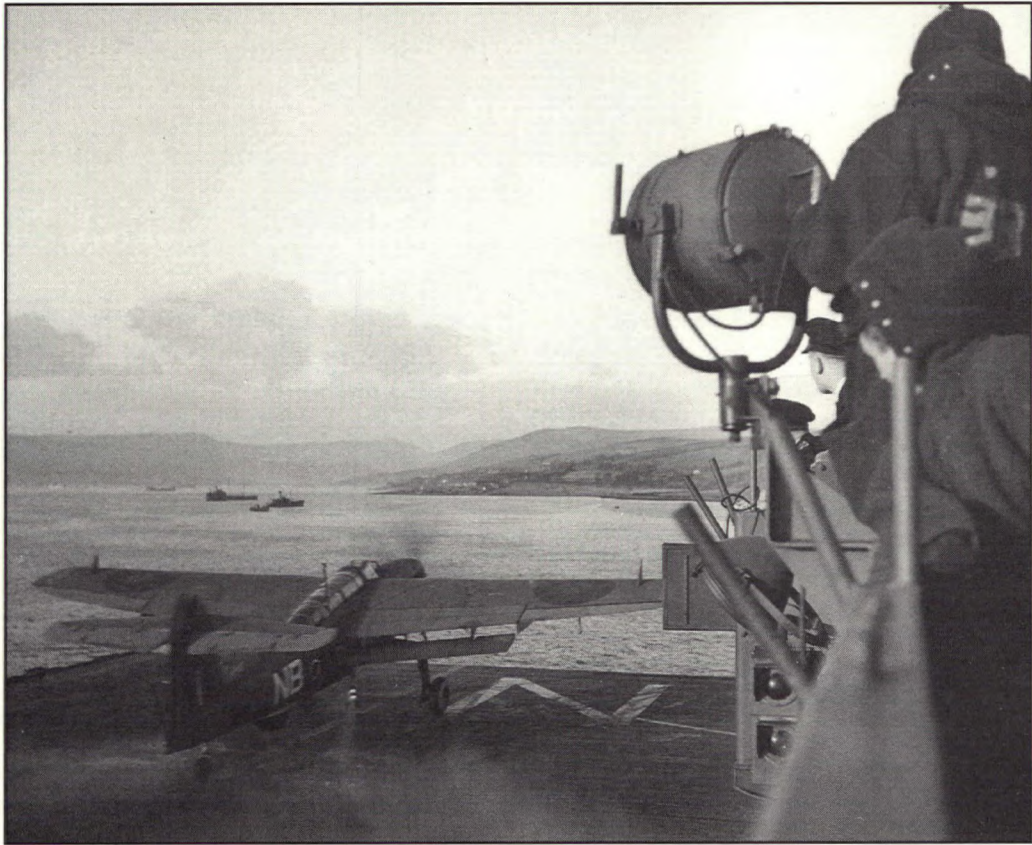
A Fairey Barracuda torpedo-bomber of 821 Squadron takes off from Puncher's flight deck. The carrier is at anchor and the Barracuda is utilizing a rocket-assisted take-off to get aloft. (DND HN-2048)
