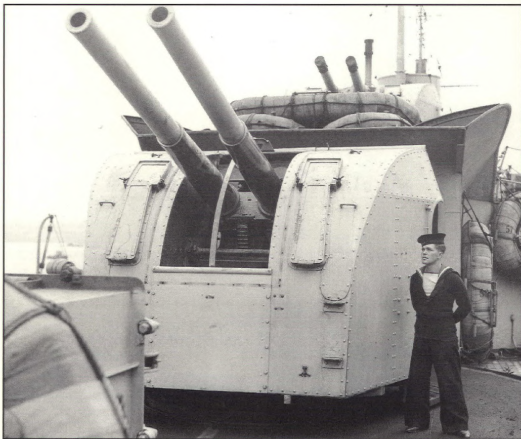
Twin 4-inch anti-aircraft guns in the former armed merchant cruiser HMCS Prince Robert . Because of the importance of air power in the Pacific, the ship would be sent there, though not in time to see action. (DND K-81)
