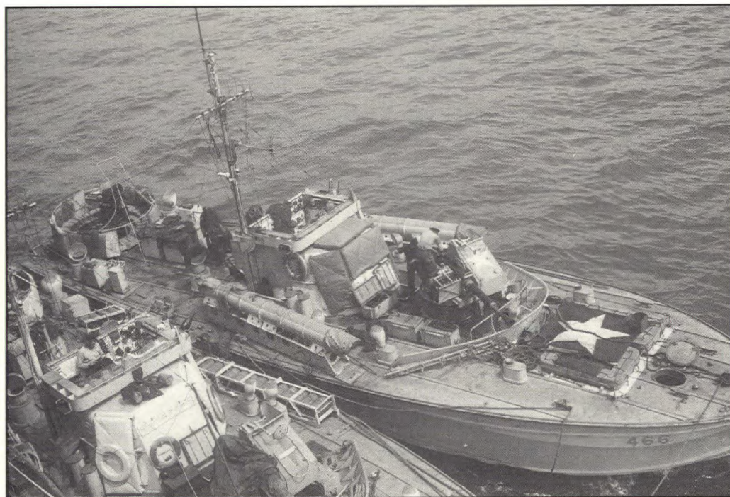
Two MTBs of the RCN's 29th Motor Torpedo Boat flotilla in the summer of 1944. Note that while MTB 466 (top) has had her torpedo tubes returned, the other boat still carries the depth charge racks, which, much to the flotilla's chagrin, were fitted to counter fast German midget submarines that never proved a reality. (DND JT 309)
