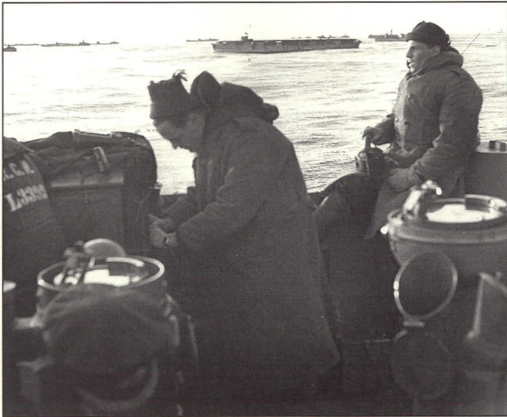
Signalling on the bridge of the River class destroyer HMCS Ottawa (2nd of name). The open bridge was designed more for open observation than for protection against the elements. A merchant aircraft carrier, or MAC ship, is in the background. (LAC PA 206691)
