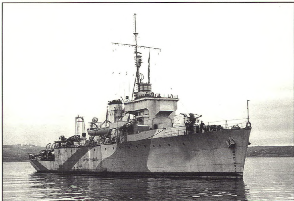
Top: The Castle class corvette HMCS Humberstone . Armed with the squid ahead-thrown weapon and modern sensors, she was one of the most advanced anti-submarine vessels in the RCN. (DND Z-1577)
