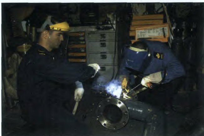
Routine maintenance carries on, whether a warship is on patrol in the Arabian Sea or off the Grand Banks. In the first photograph, Leading Seaman Brian Perry (left) and Master Seaman Stephan Pageau weld a repair to the main feed line for Charlottetown's port main lube oil system. The next photo shows that same main feed line being reinstalled the next day by (back to front) Leading Seamen John Allen, Rick Macpherson, and Eric Thibault. (HMCS Charlottetown photos, HSCHAD011202-28 and HSCHAD011203-08)
