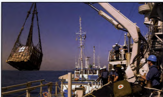
Leading Seaman J. Chaisson uses a fitted crane to sling supplies aboard Regina from a barge contracted by the Forward Logistics Site. (HMCS Regina photo by Master Corporal Frank Hudec, IS2003-2219a)
