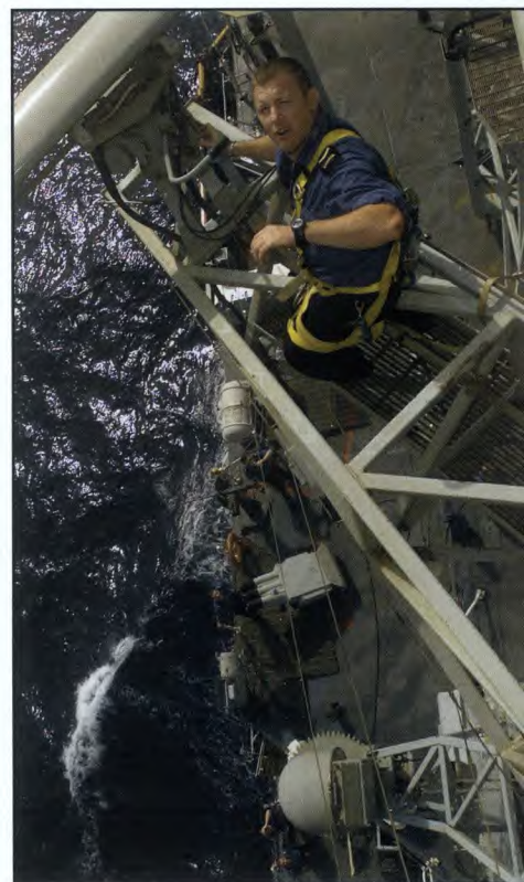
Leading Seaman Mike Coggins perches on the mast high above the bridge of HMCS Fredericton to repair the navigation radar. (HMCS Fredericton photo by Cpl Mike Selig, HS032565d15)
