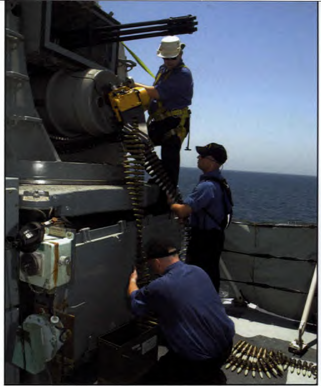
Naval weapons technicians from HMCS Ottawa replace 20mm tungsten ammunition on the Phalanx close in weapons system (CIWS), for defence against 'conventional' air and missile attack. (HMCS Ottawa photo by Cpl Charles Barber, AP2002-E018-20a)
