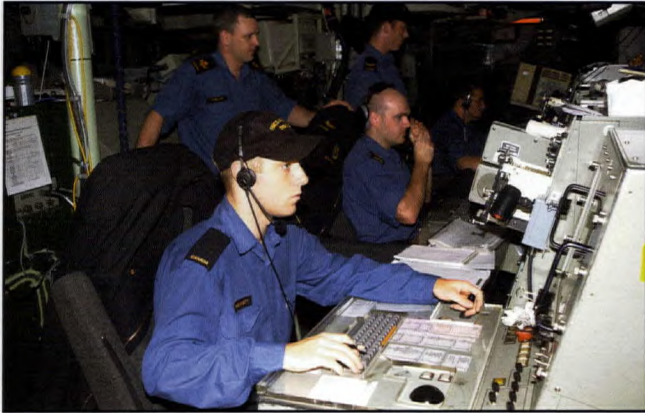
A variety of consoles in the Operations Rooms of Canadian warships display a high-tech 'fusion' of processed radar imaging overlaid with graphics generated by inter-ship datalink (computer-to-computer exchange), all representative of the unique connectivity with American and allied warships. Above left, Ordinary Seaman Wes Bennet (near) and Leading Seaman Beaumont at their radar displays in Algonquin's Ops Room; while above right another operator is 'closed up' during an Action Stations drill. Below is one of the newest displays, presenting information in a web-based format. (Canadian Forces Photos, top left AP2002-E027-71a, top right ISD01-9605a_L, below HS040161d02).
