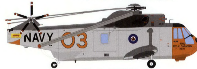
Sikorsky CHSS-2 Sea King 267 km/h - 16.7 m x 19 m x 5.13 m - 5,382 kg HS 50, NCSM Bonaventure , 1965
