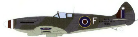
Supermarine Seafire Mk XV 594 km/h - 9.8 m x 11.2 m x 3.3 m - 2,267 kg 803 Squadron, NCSM Warrior , 1946
