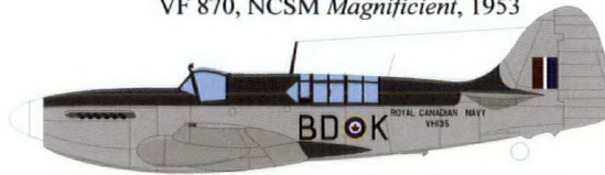
Fairey Firefly AS 5 618 km/h - 11.8 m x 12.6 m x 4.4 m - 4,472 kg 825 Squadron, NCSM Magnificent , 1950
