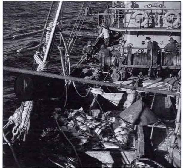
Deck scene on a side trawler. They gradually took over from schooners; then stern-ramp trawlers took over from the sides. (National Film Board)
