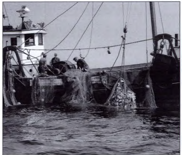
Side trawlers were still active, but giving way to stern trawlers and druggers. Photo is off Souris, P.E.I., in 1977.
