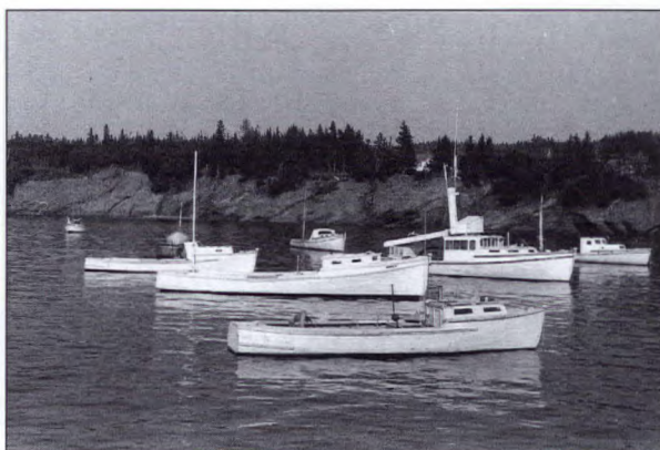
Smaller boats were still plentiful, as in this 1961 photo at Maces Bay on New Brunswick's Bay of Fundy shore, but the trend was to bigger craft. Most of those shown here fished lobster. The boat with a sluice-tank on top was a pumper for the herring-weir fishery; the pump stripped off the herring scales for separate commercial use.
