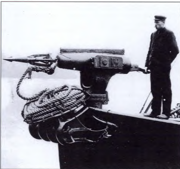
Harpoon gun on a British Columbia whaling steamer. (Library and Archives Canada, PA-40995, detail)
