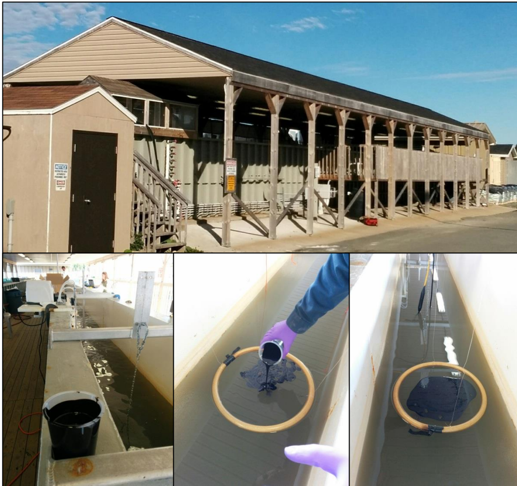
Figure 1: (a) Wave tank facility at Bedford Institute of Oceanography; (b) sediment mixing, before oil is added (dilbit sample in foreground); (c) spilling the oil, and (d) spilled oil within the containment ring, prior to wave action.
