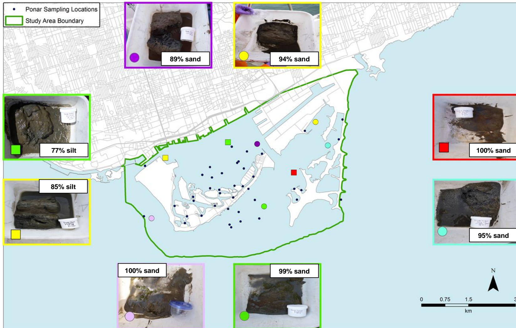
Figure 4. Locations and examples of geo-referenced Ponar sample photos taken during the 2012 Toronto Harbour survey. Includes the percent composition of the dominant sediment as determined by the Environment Canada sedimentology lab.
