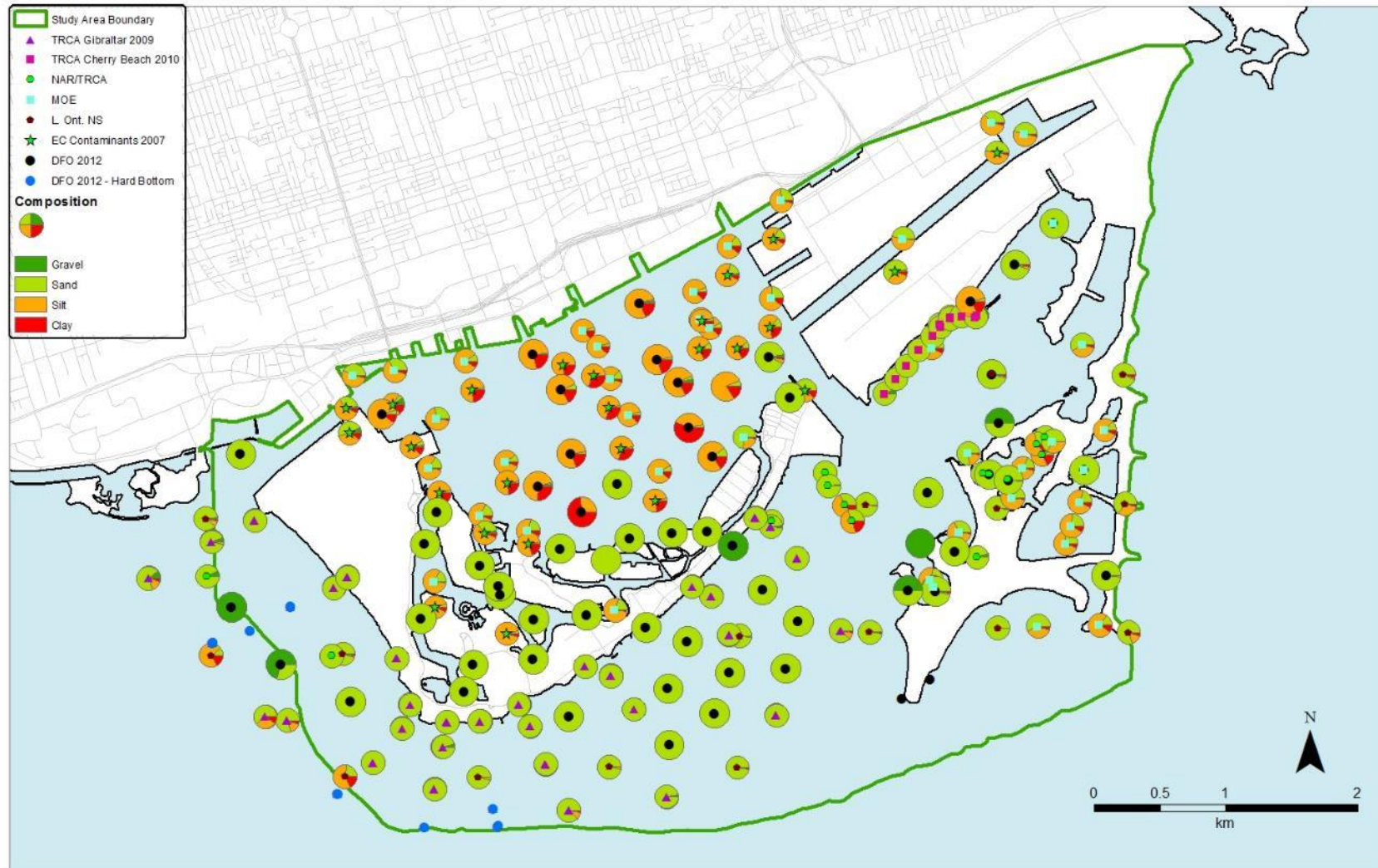
Figure 10. Sediment sample analysis results showing substrate composition of Ponar grab samples from the DFO 2012 survey (larger pie charts) and other agencies (smaller pie charts) that had sampled in previous years. The bottom was too hard to sample with the Ponar on six of the sites in the 2012 DFO survey.
