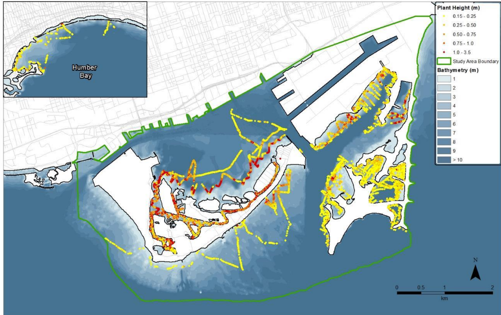
Figure 15. Submerged aquatic vegetation height as determined by the analysis of hydroacoustic data from the Toronto Harbour 2012 survey. Water depths are referenced to International Great Lakes Datum 1985.
