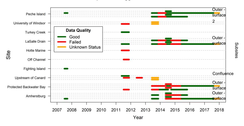
**Figure 3.** Summary of long-term temperature deployments and quality of data retrieved in the Detroit River from 2007–2018. Overall, the sites are listed from upstream (Peche Island) to downstream (Amherstburg). Sites and subsites are delineated by dashed lines. The quality of data during the duration of the logger deployment is indicated by colour.
