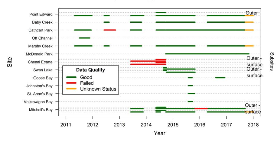
**Figure 5.** Summary of long-term temperature-logger deployments and quality of data retrieved in the St. Clair River from 2011–2018. Overall, sites are listed from upstream to downstream: from Point Edward down to McDonald Park in the St. Clair River; Swan Lake to Volkswagon Bay in the St. Clair delta; and then into Lake St. Clair (Mitchell's Bay). Sites and subsites are represented by dashed lines.
