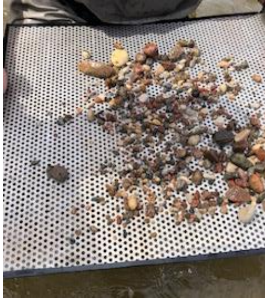
Figure 5. Metal sheet with 4.75 mm holes used to sift through pebble for mussel sampling. Approximately 40 cm of bottom substrate is shoveled onto the metal sheet. The pebbles remaining on the sheet are inspected for Zebra Mussels ( Dreissena polymorpha ). Any Zebra Mussel found is placed in a bag and transferred on ice.
