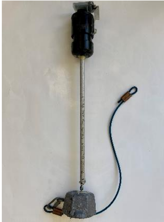
Figure 1. Wave logger set-up. A HOBO® Pendant G data logger is attached to the top of a float, created from ABS pipe, that is attached to a 4.5 kg anchor with a rigid tether on a swivel.
