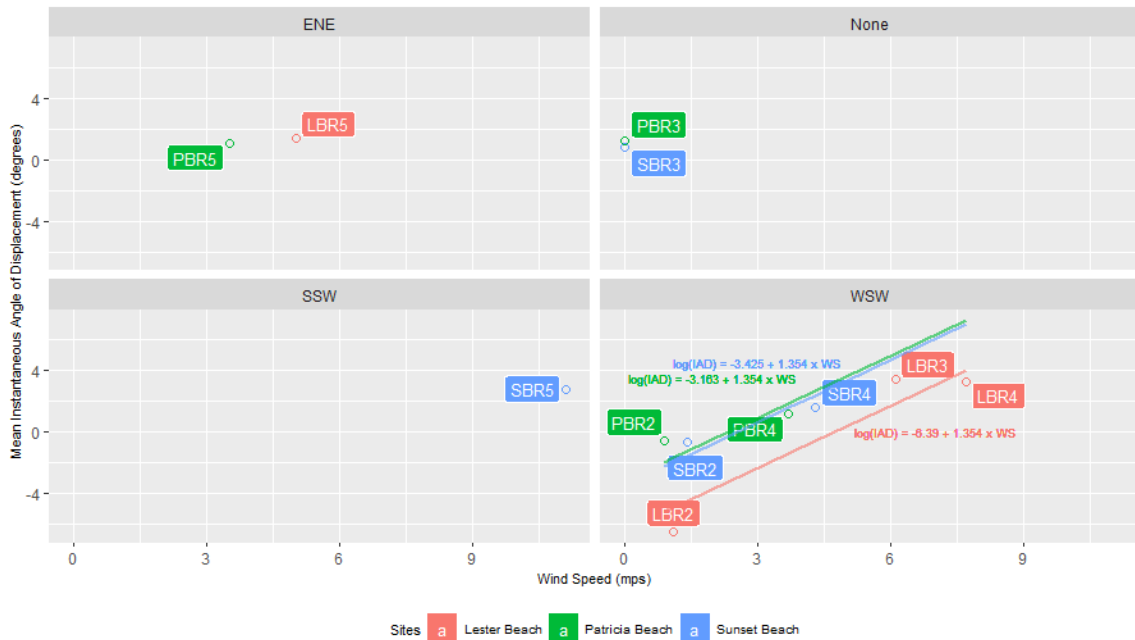
Figure 8. Mixed linear model with fixed intercept relationship between wind speed ( WS ) and mean instantaneous angle of displacement ( IAD ) calculated from initial hour of nine record periods at the summer 2019 Lake Winnipeg sampling locations for four different wind conditions, i.e., wind from east-northeast direction (ENE), no wind (none), south-southwest direction (SSW), and west-southwest direction (WSW).
