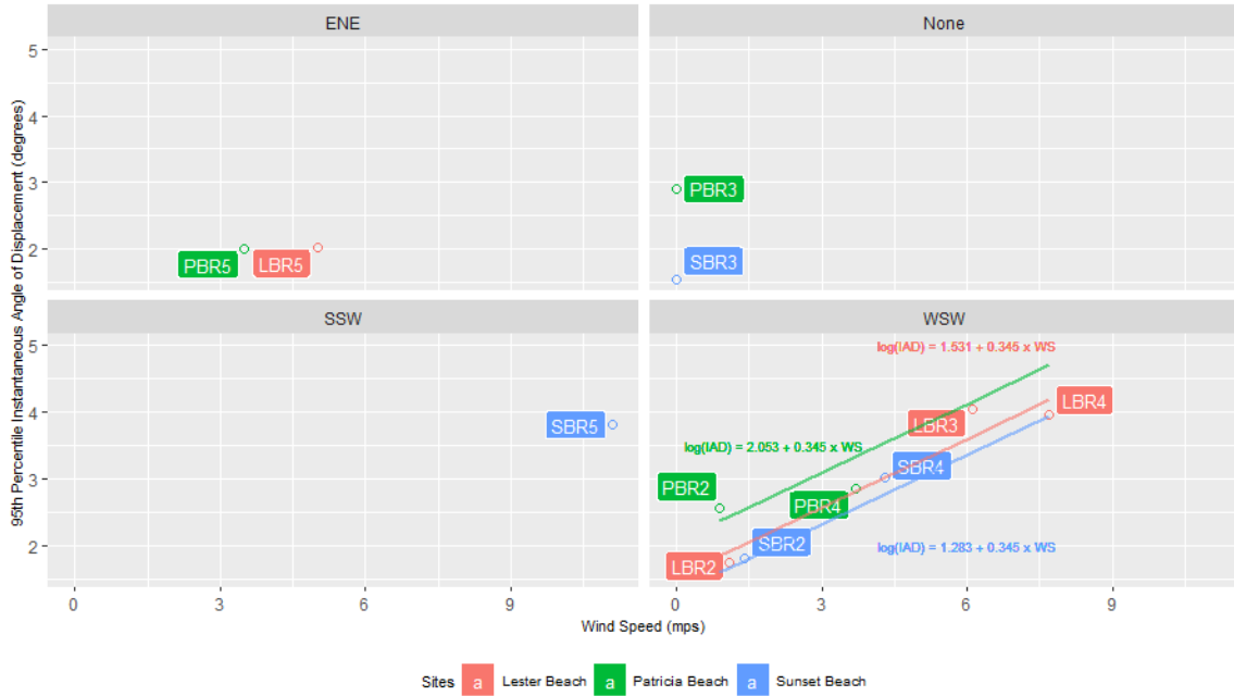
Figure 7. Mixed linear model with fixed intercept and random slope relationship between 95 th percentile instantaneous angle of displacement ( IAD ) and wind speed ( WS ) calculated from initial hour of eight record periods at the summer 2019 Lake Winnipeg sampling for four different wind conditions, i.e., wind from east-northeast direction (ENE), no wind (none), south-southwest direction (SSW), and west-southwest direction (WSW).
