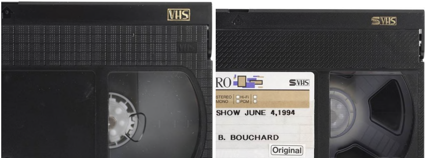
© Government of Canada, Canadian Conservation Institute. CCI 124014-0021 – CCI 124014-0020 Figure 2. VHS cassettes can be distinguished from S-VHS cassettes by looking for the stamped logo found at the top right corner on the front of the cassette housing.
