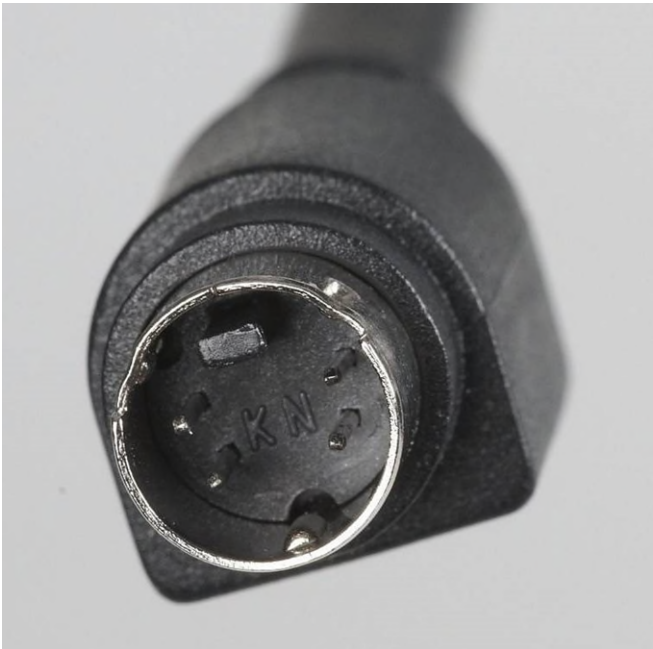
© Government of Canada, Canadian Conservation Institute. CCI 124014-0013 Figure 13. Close up of an S-video cable showing the 4-pin configuration.
