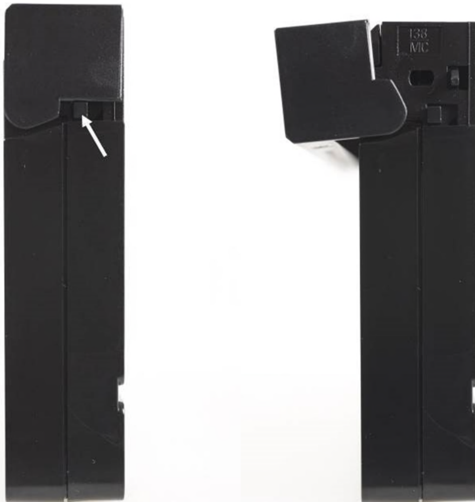
© Government of Canada, Canadian Conservation Institute. CCI 124014-0023 – CCI 124014-0022 Figure 5. Left image: Pressing the button indicated by the arrow allows the spring-loaded gate to be manually opened so that the proper functioning of the gate can be verified. This is an essential component of the cassette. Right image: The same cassette with the gate opened.
