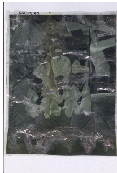
Figure 9. Cellulose acetate negative sheet at an advanced stage of degradation, also due to hydrolysis. The film base is yellow and very brittle.
