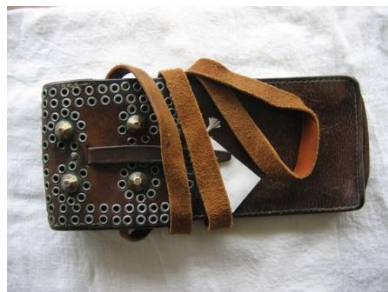
Figure 7. Copper in contact with a greasy leather forming a waxy green copper corrosion compound: copper stearate; this is an example of an intrinsic pollutant.
