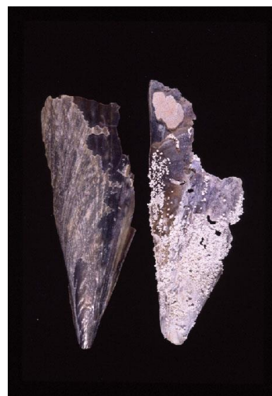
Figure 6. Efflorescence on shells. The shell on the right has been exposed to a high concentration of acetic acid vapour.
