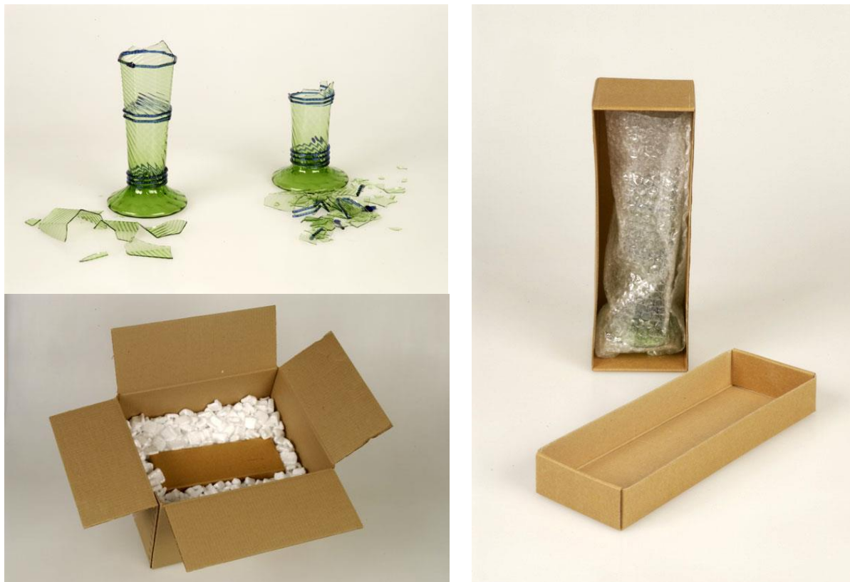
Figure 14. Reproduction glasses made of soda lime glass. Individual boxes containing loosely bubble-wrapped glasses moved in the peanut packaging material and collided, resulting in damage to the pieces.
