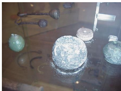
Figure 1. A lead paten or weight severely corroding, due to chipboard bottom of display case (photo courtesy of Christoph Waller).
