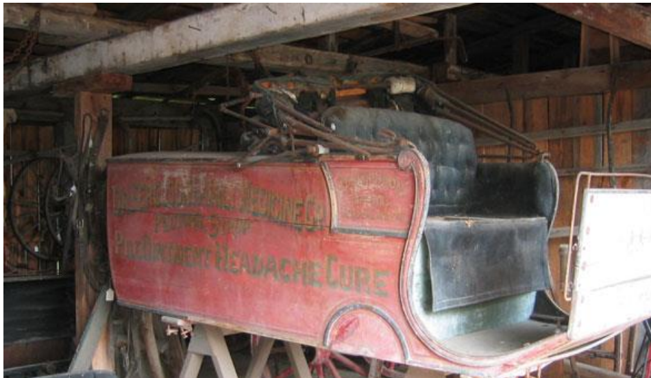
Figure 1. Image of an old horse-drawn carriage. Mould and rapid corrosion caused by damp. A thin blue green layer of mould on the leather seats, and deep rusting of all the iron components, is typical in a shed that is dry most of the year, but damp in spring and fall.
