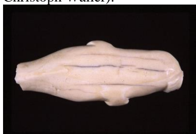
Figure 1. A lead paten or weight severely corroding, due to chipboard bottom of display case (photo courtesy of Christoph Waller).
