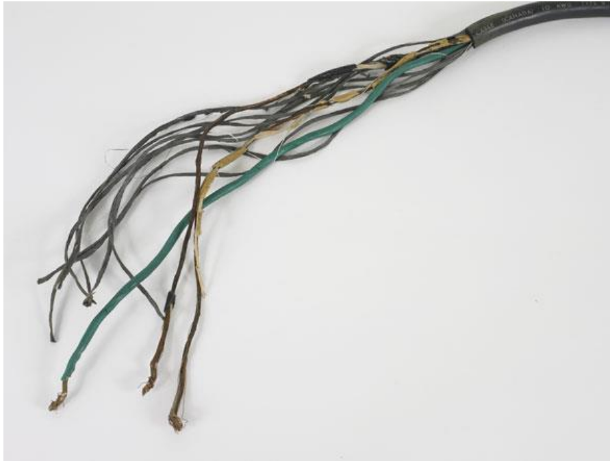
Figure 3. The defective wiring shown here was part of a power supply cord from a laboratory oven. Have the building's electrical system inspected by an electrician at least every 10 years, maintain heating systems annually, and inspect tools, equipment, and appliances — large and small — regularly to reduce the risk of fire from electrical sources.
