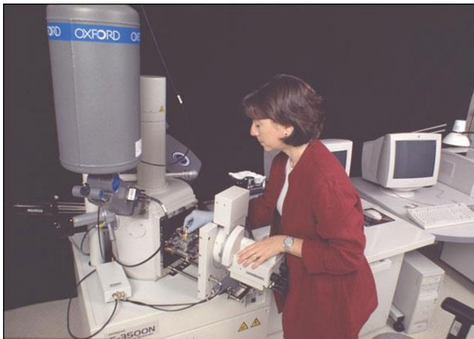
Figure 8. An electron microscope can be adversely affected by vibration levels that are far below levels that people can perceive. Other vibration-sensitive instruments, such as microscopes and precision balances, are commonly found in museums.
