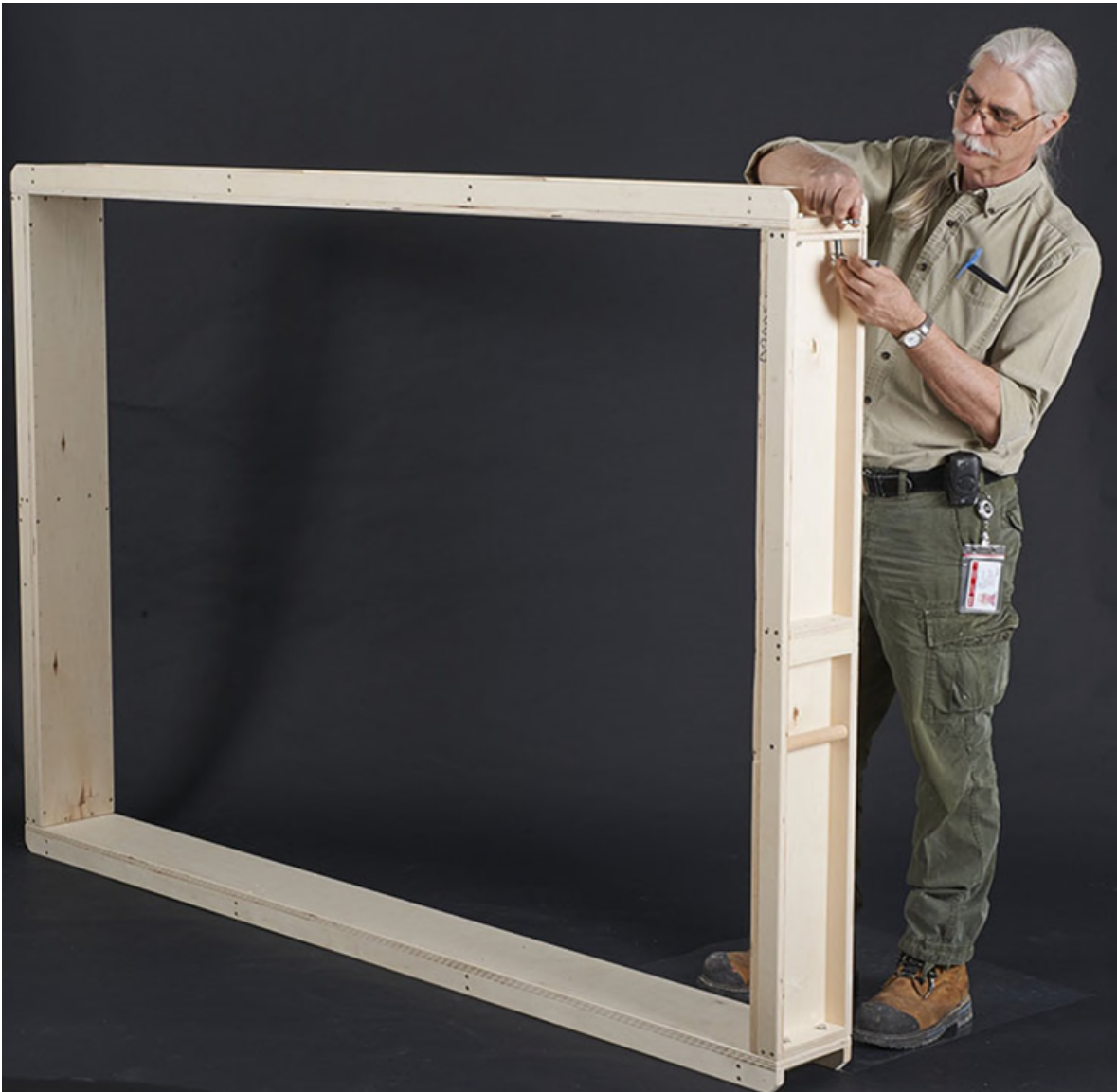
© Government of Canada, Canadian Conservation Institute. CCI 124851-0151 Figure 1. Plywood channels being assembled.
