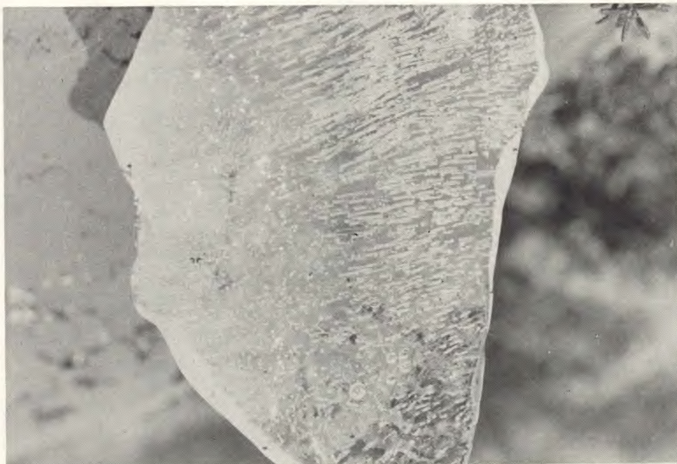
B. Close-up of the vertical cross-section of the ice wedge at site T35C. Note the bubbles and bubble trails fanning out from the centre of the wedge.
