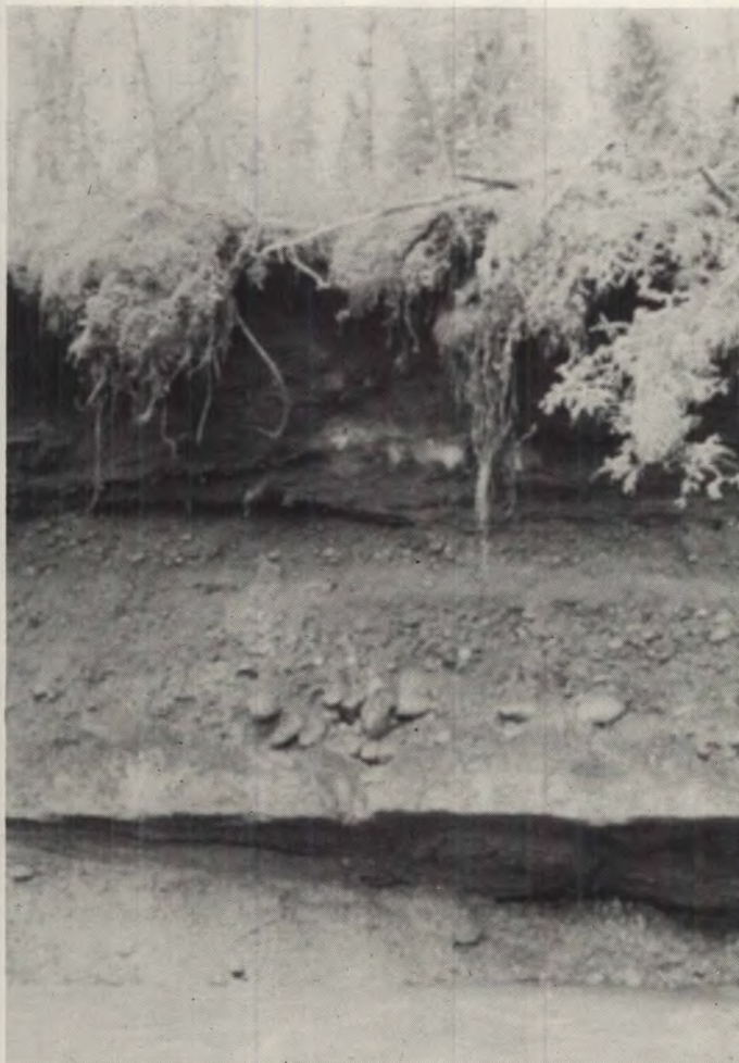
A. Vein ice in fine textured till at a depth of 55 cm. The ice content of this depth was found to be 58 percent on a weight basis. Southwest side of the Wrigley Sheet.
