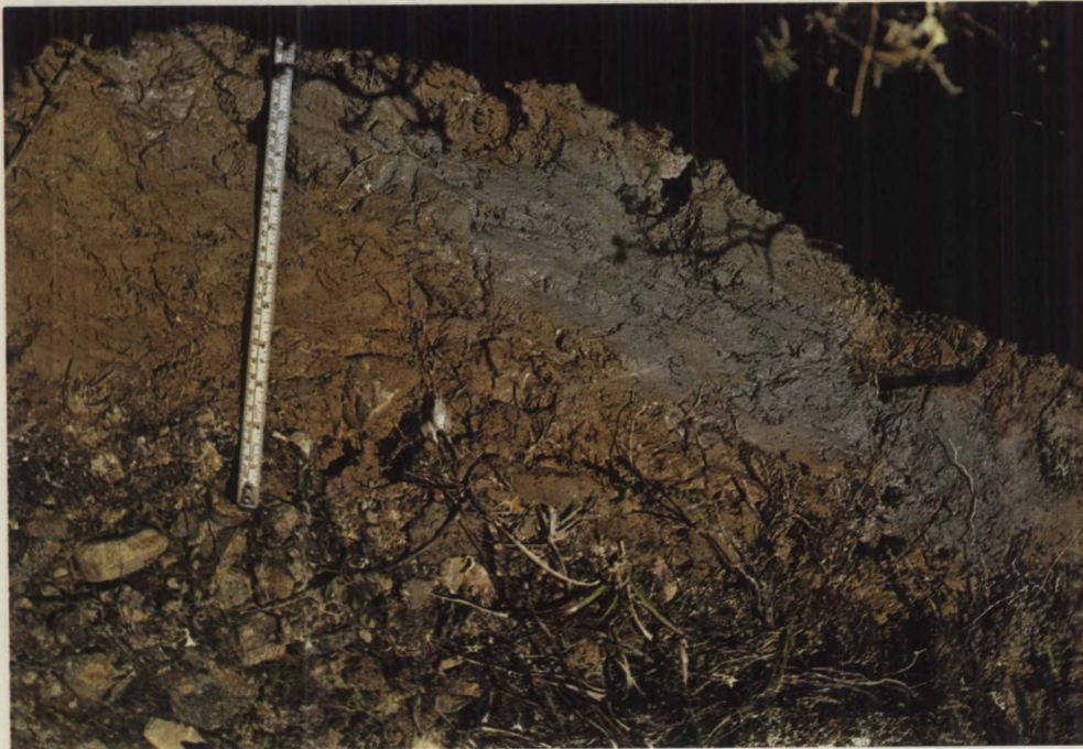
A. Extremely cryoturbed Cryic Orthic Dystric Brunisol developed on unglaciated terrain in the Mackenzie Mountains. Note the displaced B and C horizons. Profiles ZT8A and B, located on a nonsorted circle.
