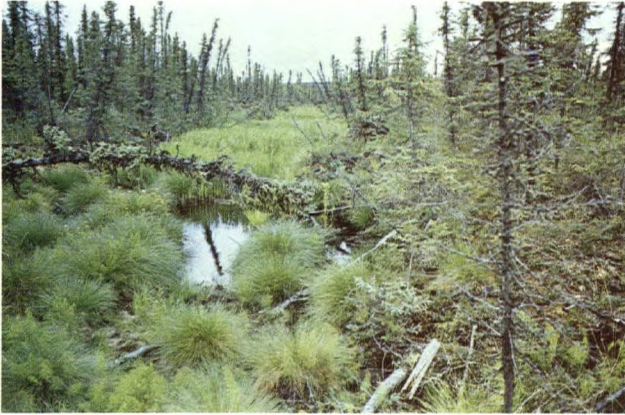
Figure 28. Old seismic line in silt with about 1 m. subsidence. Note trees leaning toward line, indicating lateral spread of thermokarst conditions. Location: Lat. 65°52'N and Long. 136°55'W
