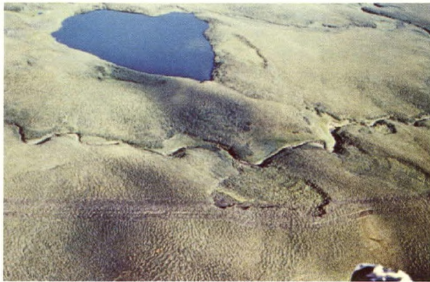
Figure 29. Old flow slide scar, flow slide partially reactivated by seismic line too close to the escarpment. Note that little reaction is shown elsewhere on the line. Location: Lat. 67°16'N and Long. 136°49'W
