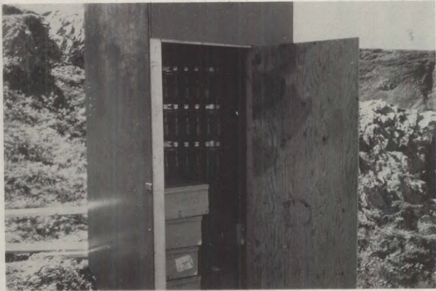
Sediment Pumping Sampler in Portable Shelter — Firth River
